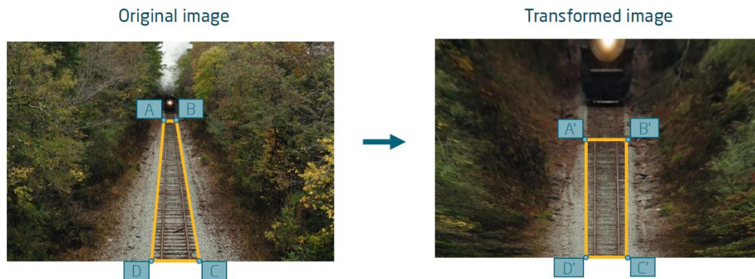
Figure 7.53 Homography transformation example.
