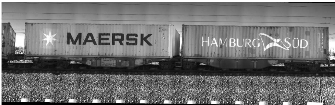
Figure 7.66 Stitching process: Panorama image of a complete wagon generated by merging multiple frames captured.
