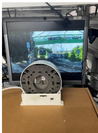
Figure 7.51 Integration test Train Detection Module detection camera.
