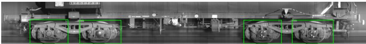
Figure 7.5 Object detection of the wheelset areas
