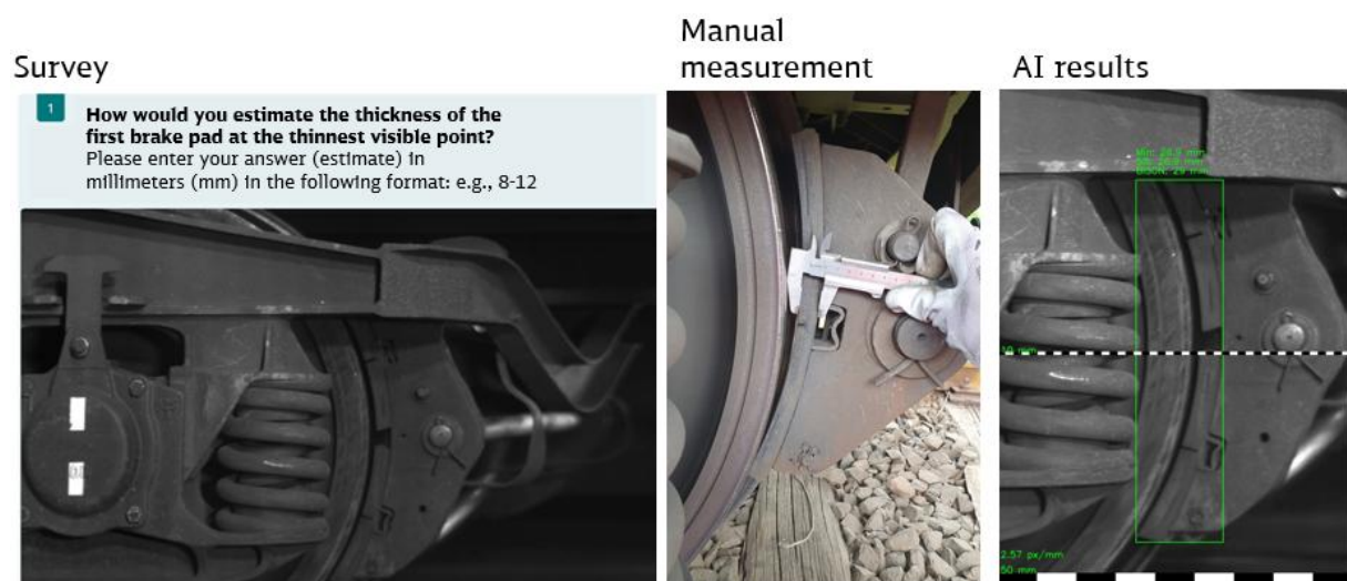
Figure 7.27 Validation approach for brake pad thickness
