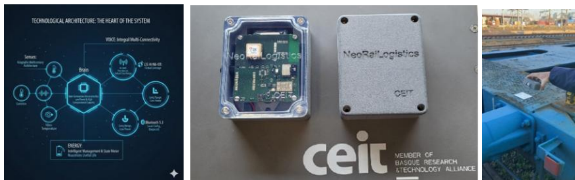
Figure 7.69 a) Field layer hardware architecture, b) CEIT's modular device for WOBUM (Wireless On-Board Unit Module), WOBUC (Wireless On-Board Unit Central), or WSEN (Wireless Sensor Elements) operation, c) Installation of an on-board unit
