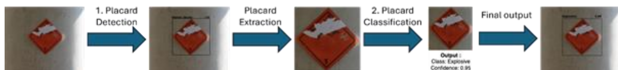
Figure 7 Overview of the automatic hazmat placard detection and classification pipeline. The first model detects the placard, predicting a bounding box around the located placard. The next step is placard extraction, after which the second model classifies the placard category. The final output consists of the bounding box indicating the location and the predicted category.
