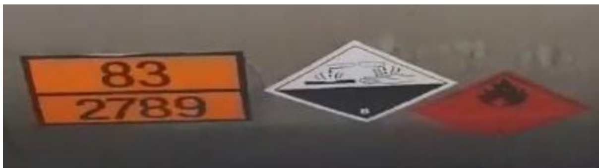
Figure 4 Example of a hazmat plate (left: the orange plate) and hazmat placards (right: the two-diamond shaped placards) – Image originates from private data collection.
