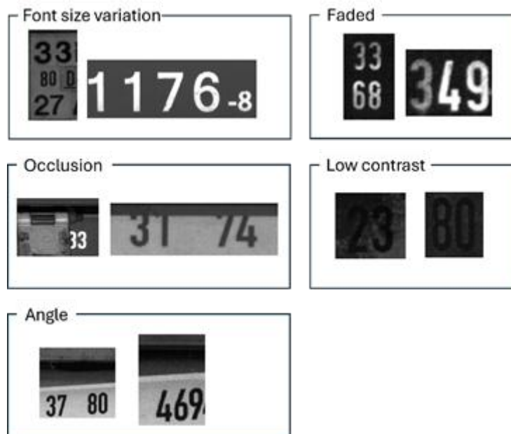
Figure 15 Examples of the 5 most common challenges found in the line-scan dataset. Only partial codes are shown.
