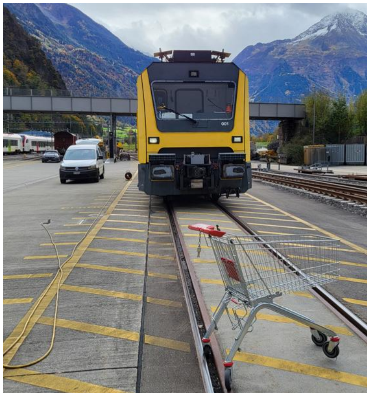
Figure 13: Example picture for test case - object on the track (trolley)
