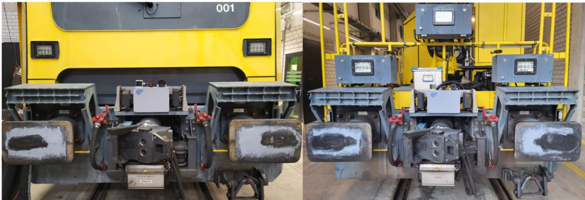
Figure 9: Position of perception system (left: frontside / right: backside)
