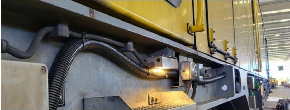
Figure 7: Example picture for final cabling outside of the vehicle
