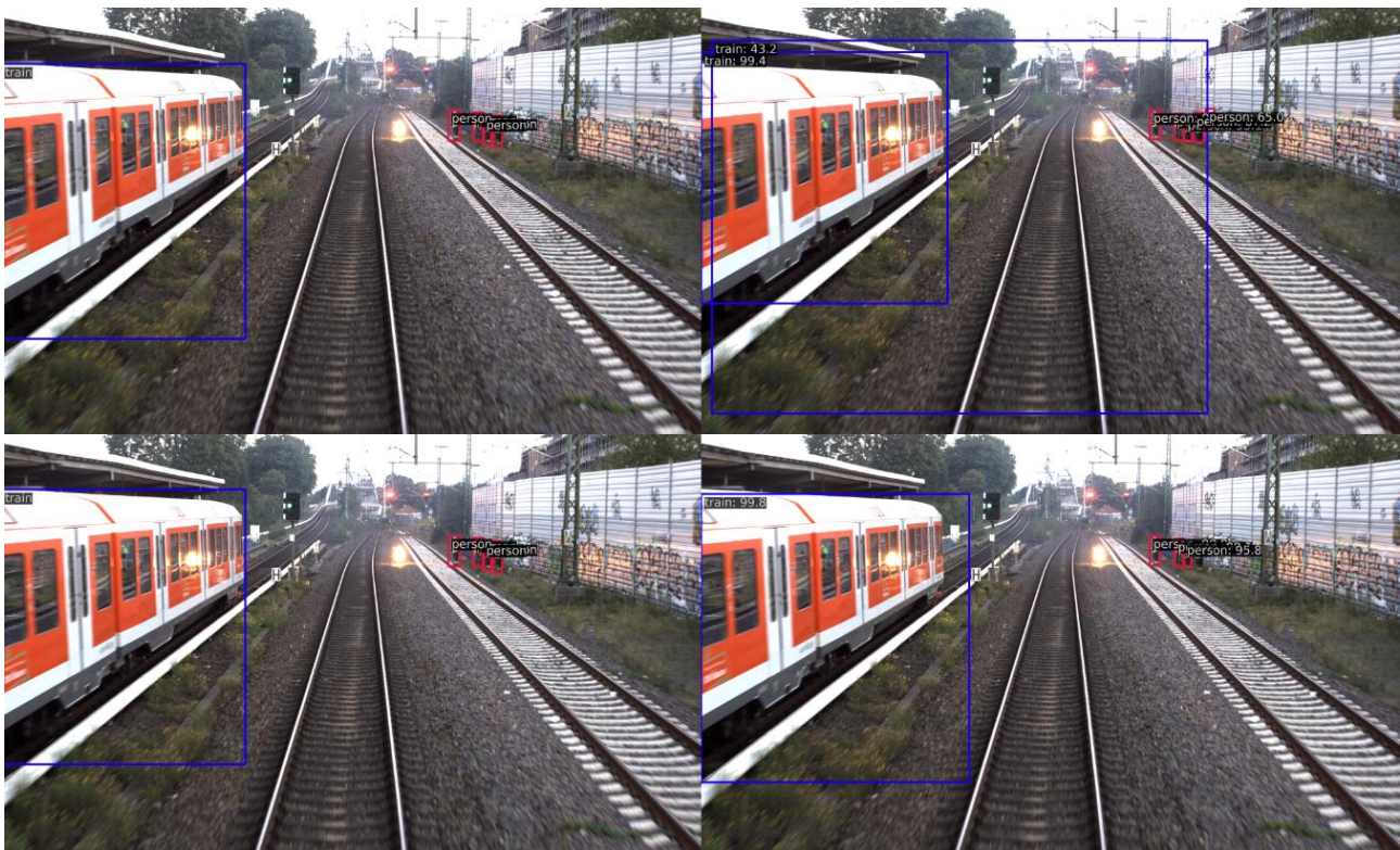
Figure 9: Exemplary detection results OSDaR23 (left: ground truth, right: detections. 1st row pre-trained model, 2nd row refined model)
