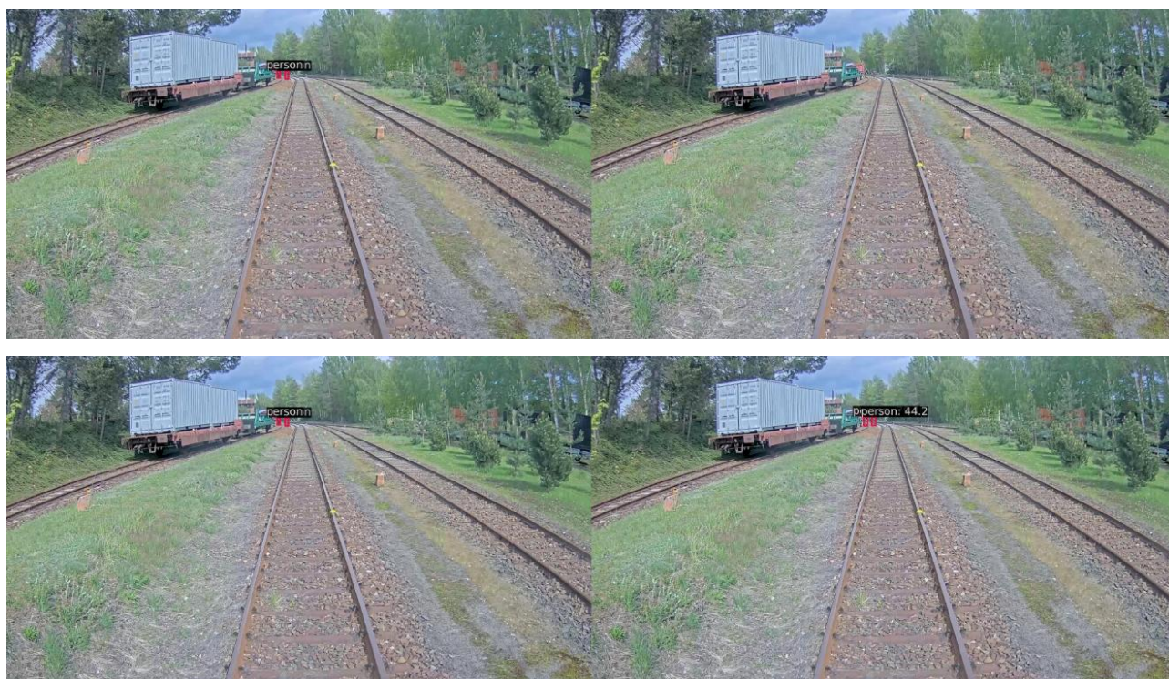
Figure 14: Example detections RailGoerl24 (person class), left: ground truth, right: detections. Pre-trained model (1st row) vs. refined model (2nd row)
