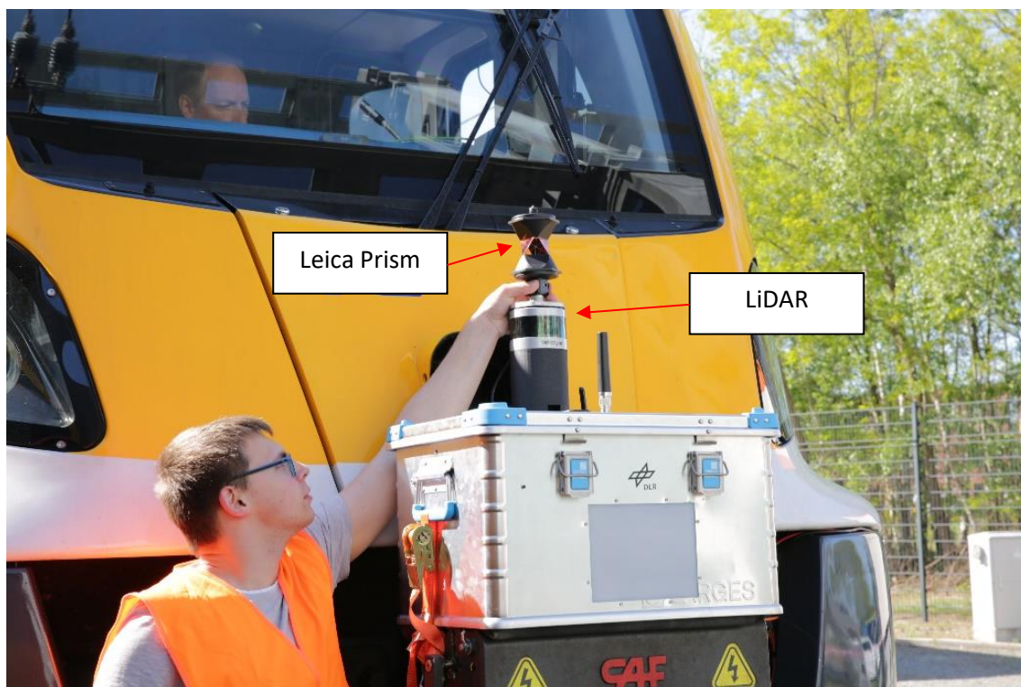
Figure 5: Ground truth LiDAR Velodyne Puck VLP-16
