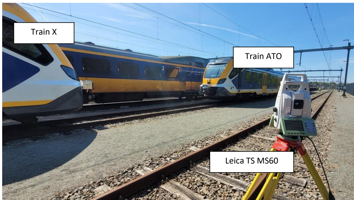
Figure 4: Ground truth Leica TS MS60
