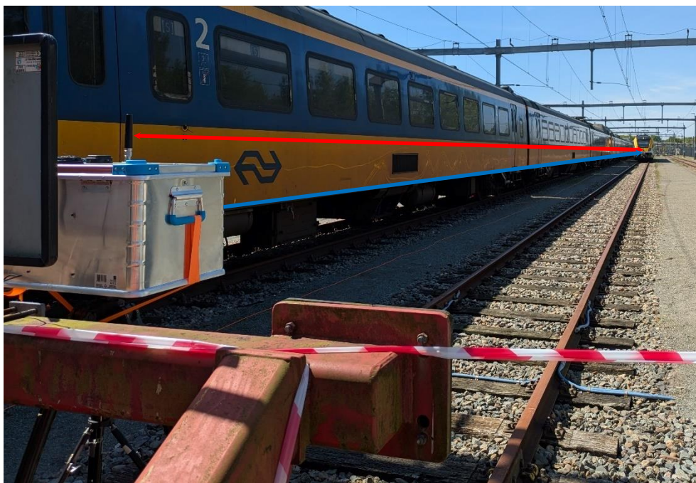
Figure 18: Indicated LoS signal of the SRC and RL measurement links with omni-directional antennas (red line) and directional antennas (blue line) on the same track (test case 1, 2, 3)
