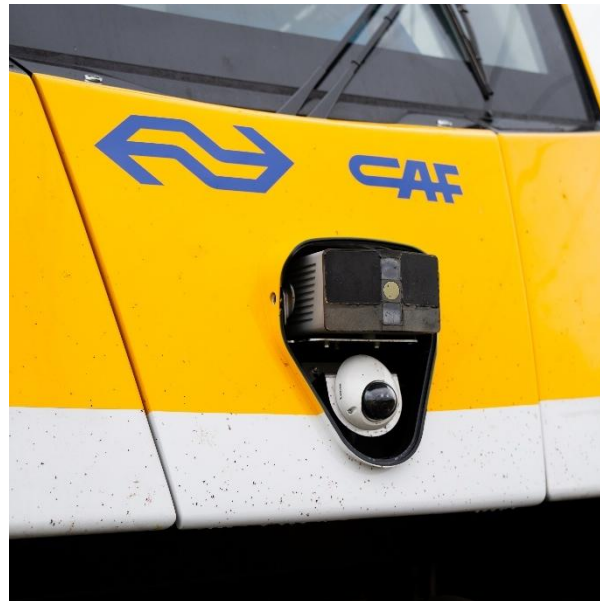
Figure 2: Sensor positions on demo train
