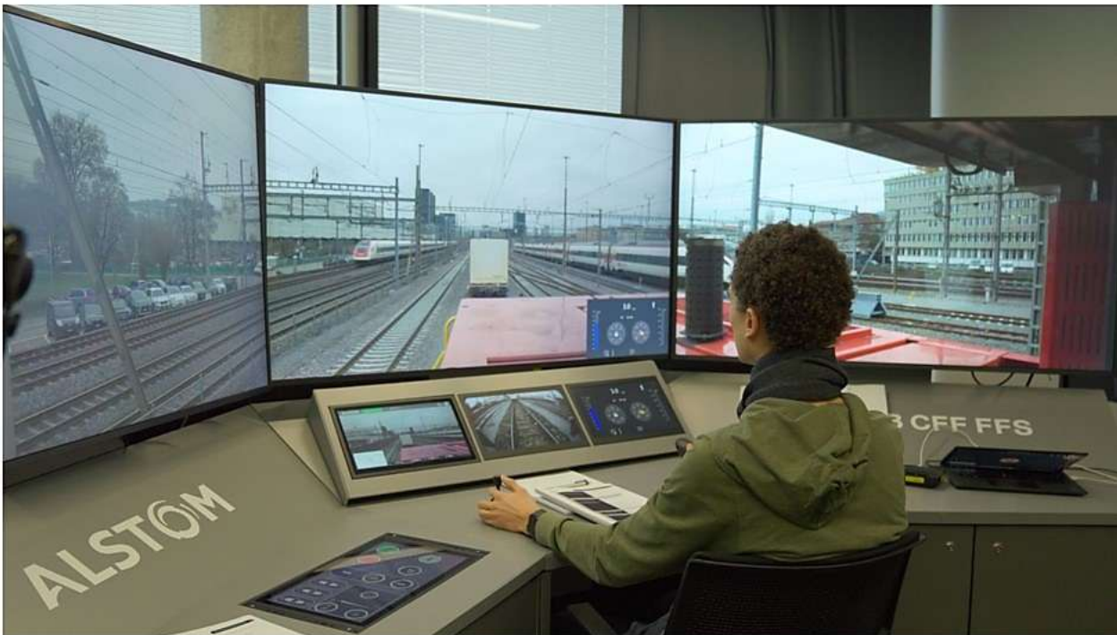
Figure 6 - Remote control desk with panoramic view during the manoeuvre
