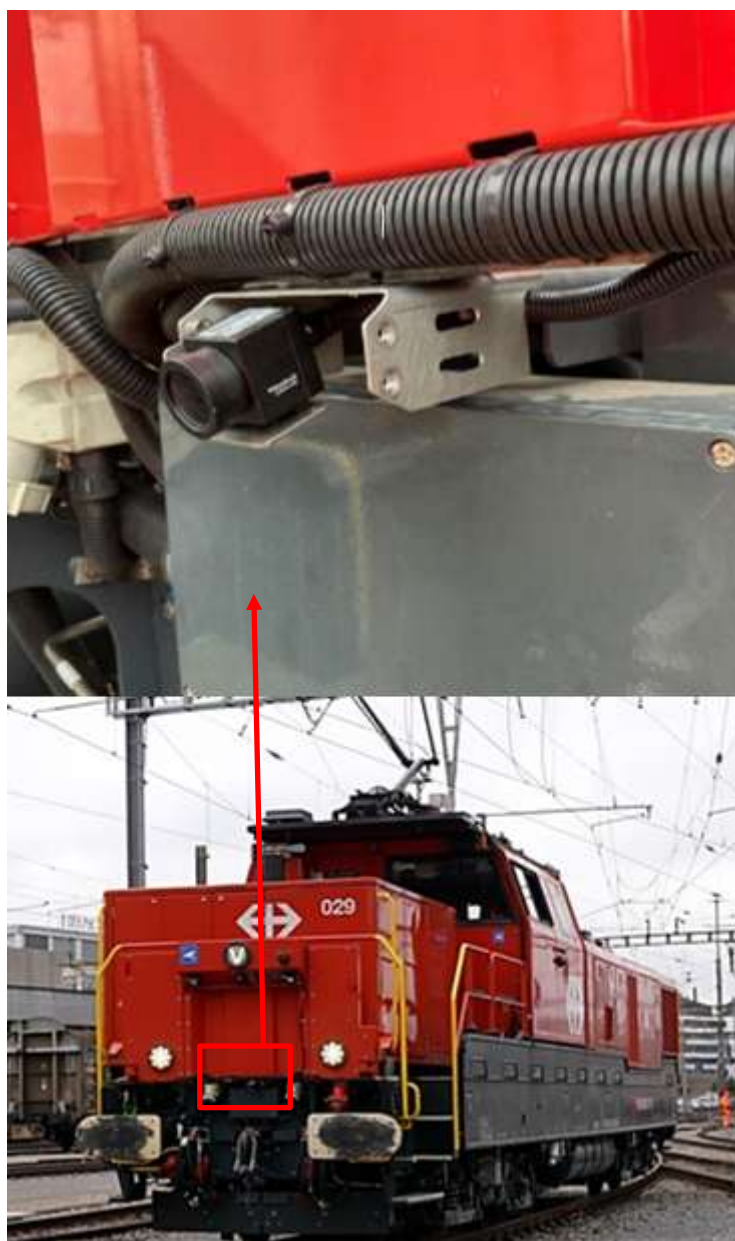
Figure 5 - Installation and arrangement of the front camera / near field camera
