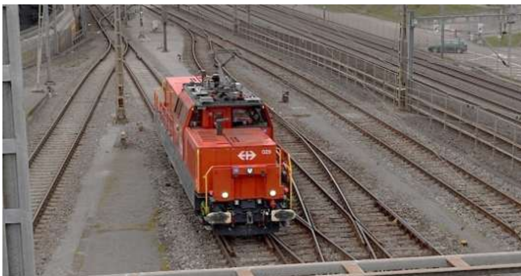
Figure 3 - Locomotive during a remote-controlled manoeuvre
