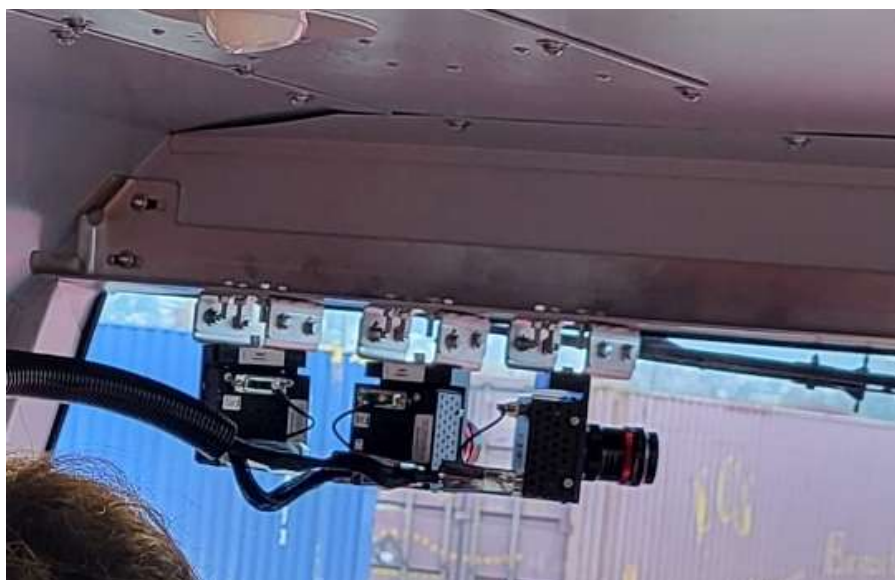
Figure 4 - Installation and arrangement of the cameras in the driver's cab
