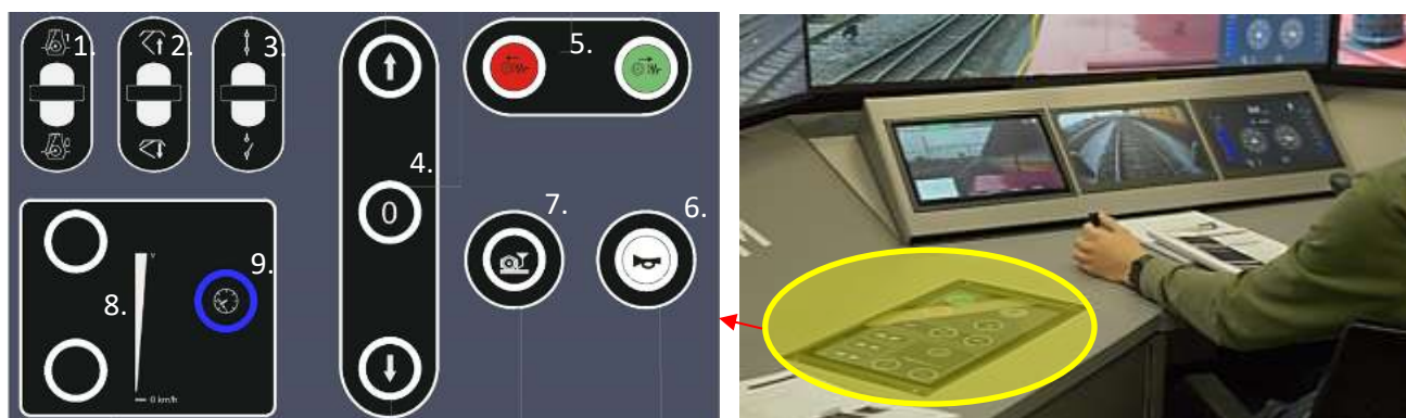
Figure 8 - Layout of control panel (left) and integration of control panel in driver's desk (right)
