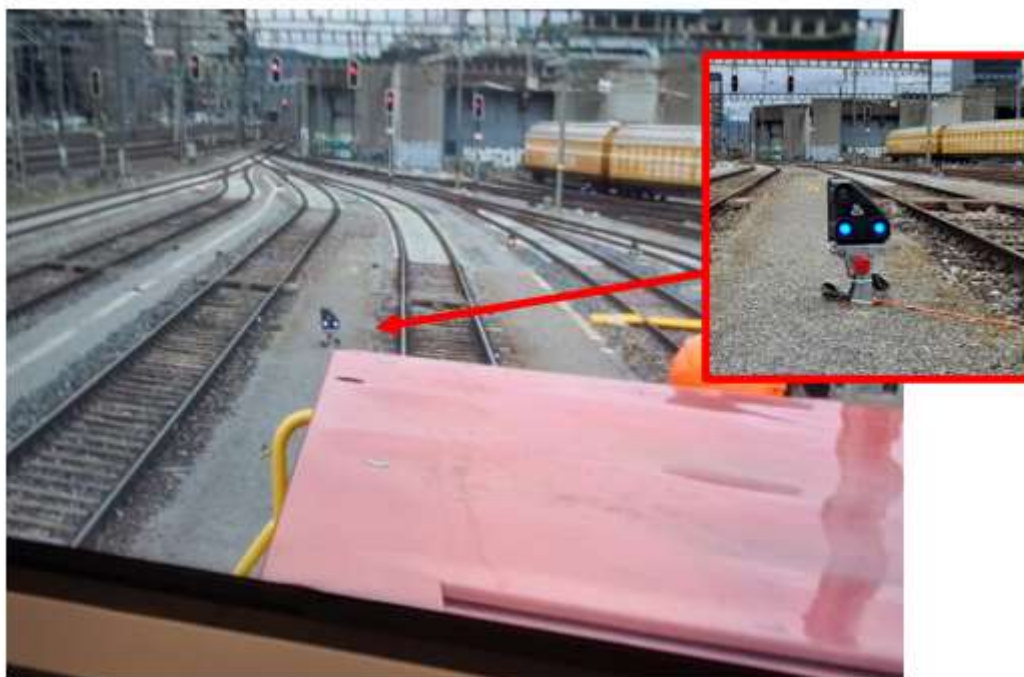
Figure 28 - View of ETCS shunting signal in "Stop" position on the remote desk
