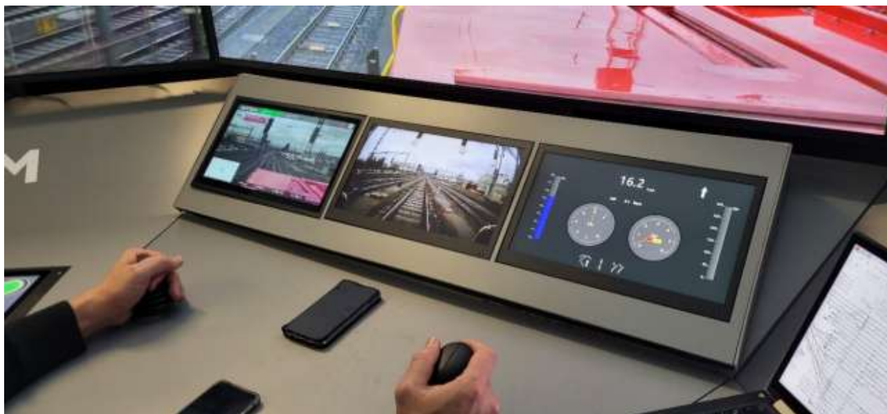
Figure 7 - Displays with driving information and video image
