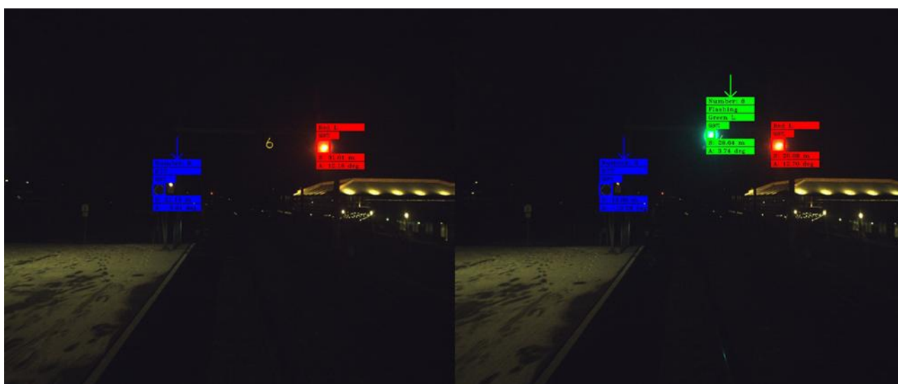
Figure 9: PER output example scene at night, with consecutive frames where the green light is blinking being off (left) and on (right). PER proposes its aspect as Flashing Green 6.
