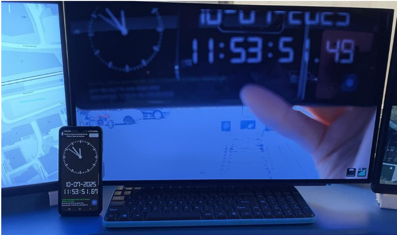
Figure 1b: Measurement using glass to glass method.
