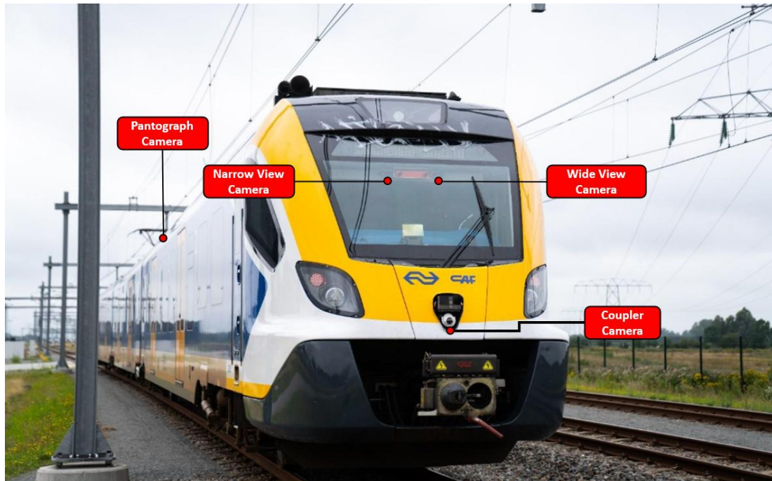
Figure 13: Physical location of RD Cameras.
