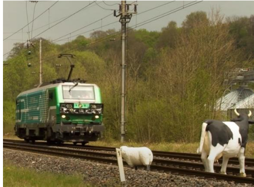
Figure 26: ATO Freight train SNCF project – obstacle detection
