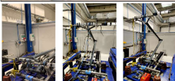
Uplift and down lift test
