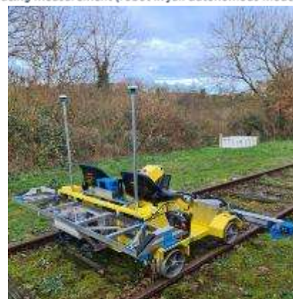
Reproducibility of rail spacing measurement (robot in full autonomous mode)
