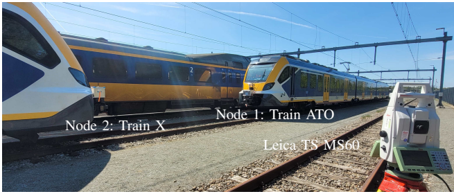
Fig. 2: Train X and Train ATO nodes mounted on the trains with Leica TS MS60 laser tracking in front.
