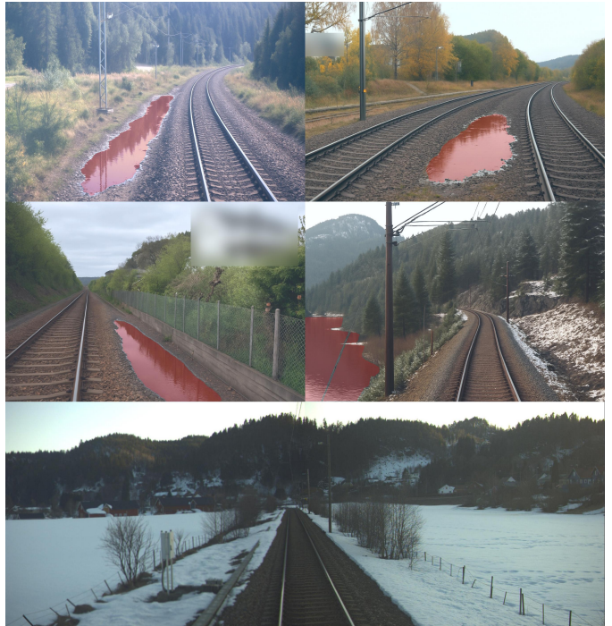
Fig. 2. The full training set with transparent red segmentation masks, top four are synthetic, while the bottom is a natural image.
