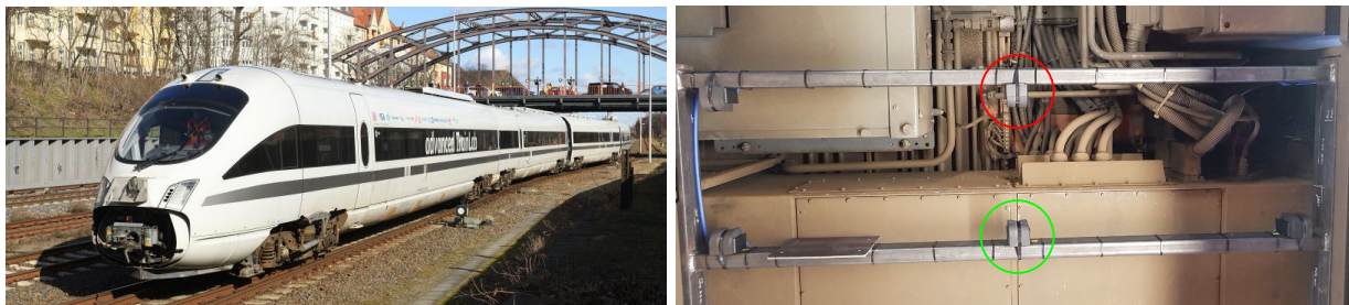
Figure 2: (left) ATL on a track in Berlin. (right) Magnetometer array with five elements mounted below a wagon of the ATL. One of the magnetometers (green circle) is used only to create the magnetic map and another sensor (red circle) is used exclusively for localization.
