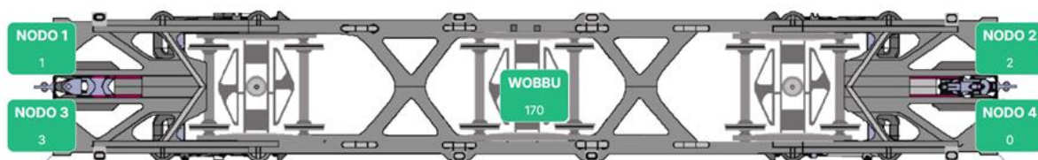
Figure 7.13 WOBUC and WSEN units within the wagon
