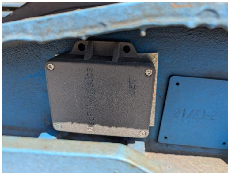
Figure 7.10 On-board unit attached to the metal plate
