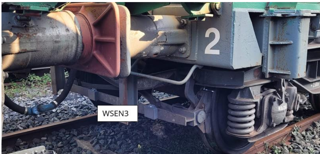
Figure 7.7 Brake beam of the brake linkage
