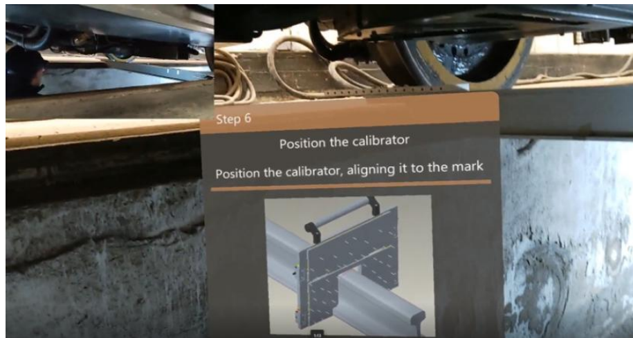
Figure 2. AR Instructions of the setup for a track measuring device
