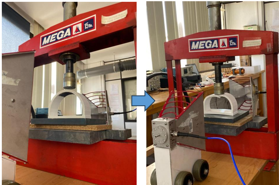
Figure 26: New prototype made with PLA in 3D printer
