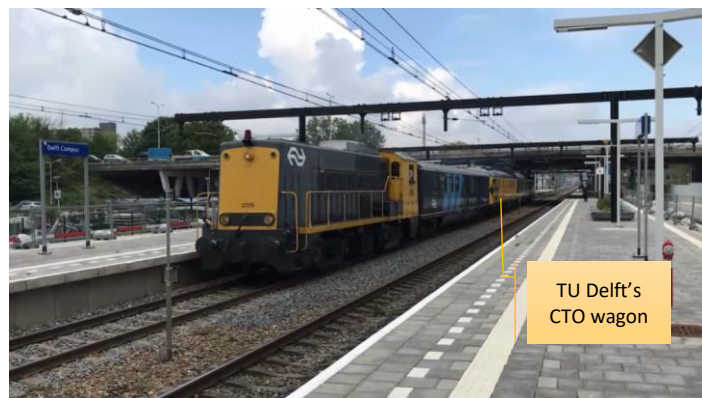
Figure 75: ABA measurement with the CTO, TU Delft's measurement wagon. The photo was taken as the train passed Delft Campus station.
