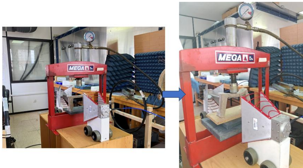
Figure 24: New load-applying press and concrete prototype
