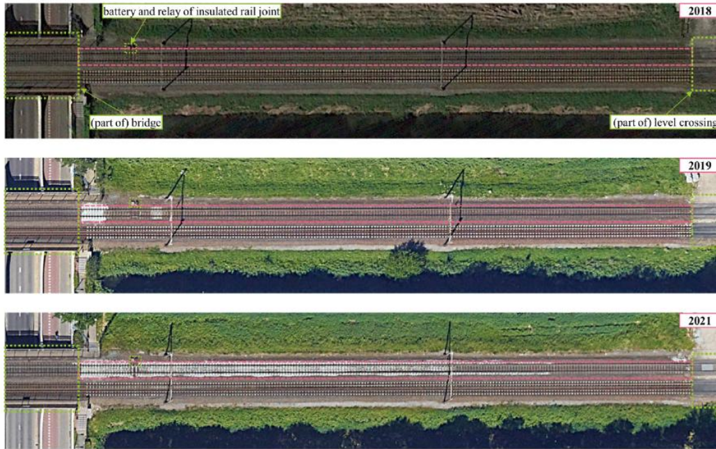
Figure 64: Historical satellite photos of an example segment for temporal consistency analysis. Changes can be seen as evidence of track maintenance activities in ballast appearance [4].
