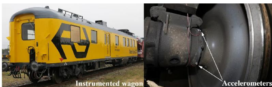
Figure 41: ABA measurement system on the CTO, TU Delft measurement wagon [1].
