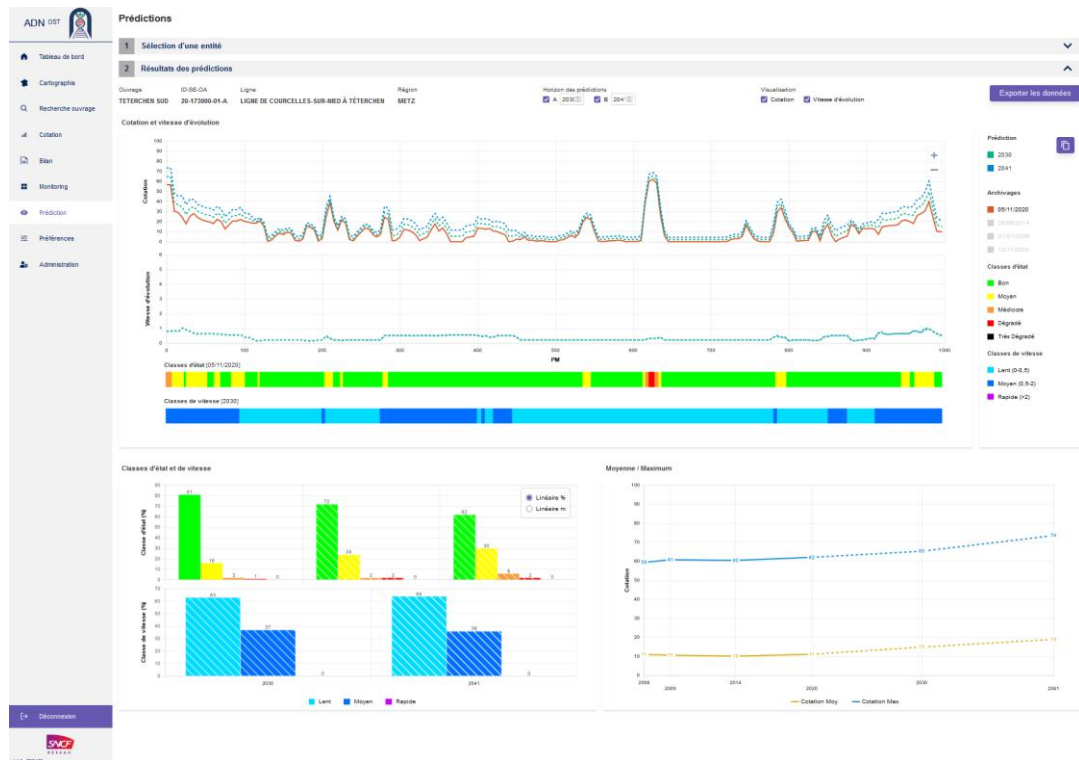
Figure 70: Predictive Degradation Modeling Interface for a Tunnel (2030 & 2041)
