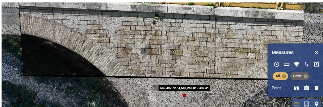
Figure 5-81: Measuring a point from the point cloud
