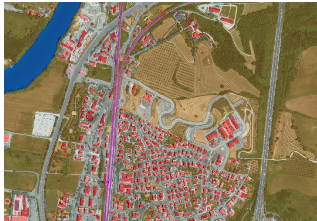
Figure 5-23: Segmentation results close-up. Blue: Seas, lakes, rivers; light brown: Groups of trees and fields; grey: Yards, technical areas and streets; red: Buildings; purple: Railway tracks.
