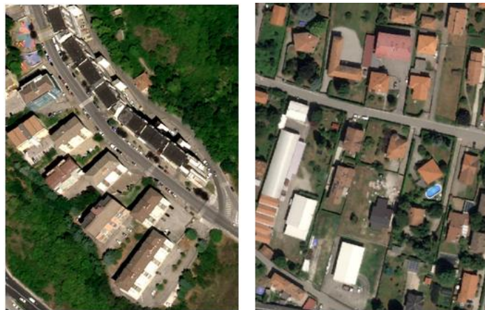
Figure 5-2: Left: piece of old data, with 19 degrees of inclination. Right: piece of new data, with 6 degrees of inclination.
