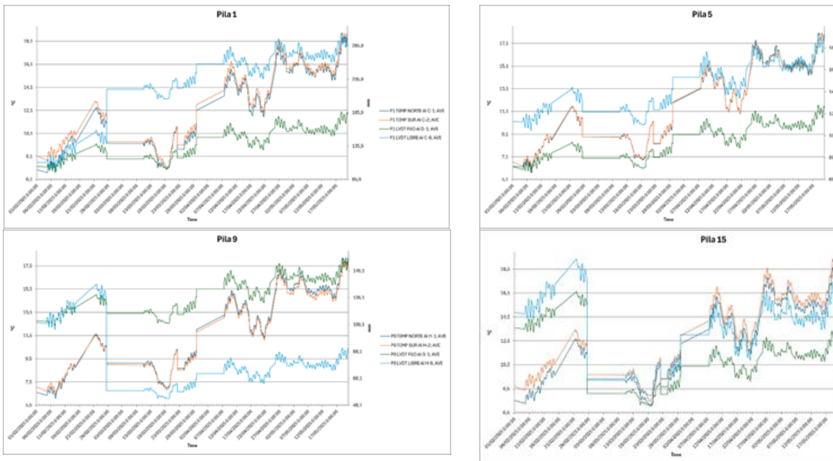
Figure 6-26: Recorded temperature and displacement data. February-May 2025.
