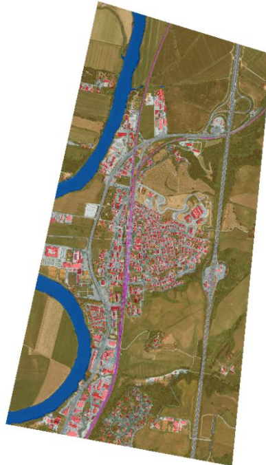
Figure 5-22: Segmentation model predictions on inference data. Blue: Seas, lakes, rivers; light brown: Groups of trees and fields; grey: Yards, technical areas and streets; red: Buildings; purple: Railway tracks.
