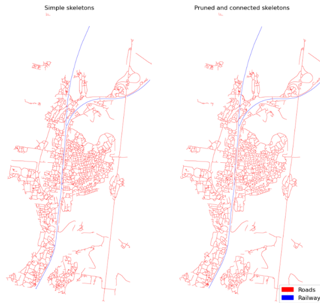
Figure 5-27: Left: original roads and railway skeletons. Right: skeletons after pruning and endpoints connecting.
