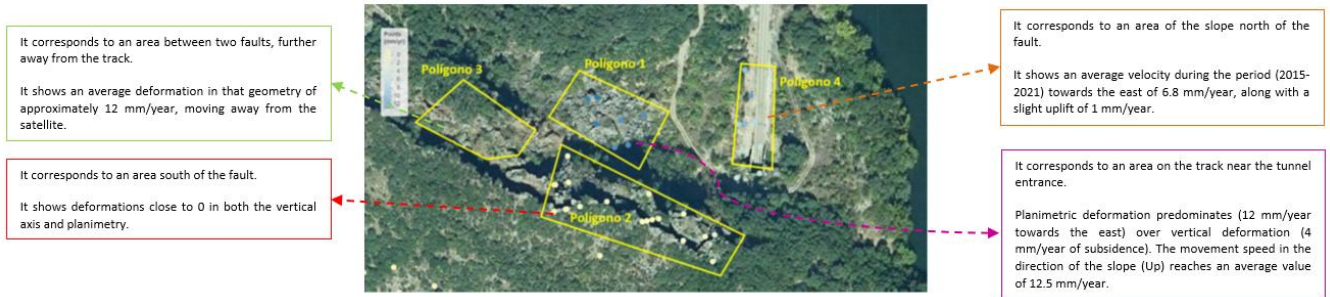
Figure 6-43: Study Area Polygons and DInSAR Measurement Density Map.
