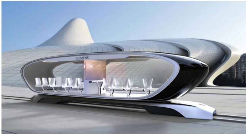
Figure 5: ANTS design study, autonomous micro-vehicle consisting of drive unit and life unit for the individualised transport of passengers (© SIEMENS AG) [6]
