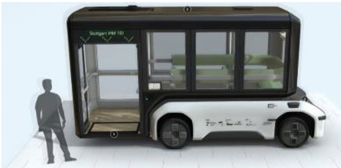
FIGURE 23. Intermodal passenger pod with road pod carrier
