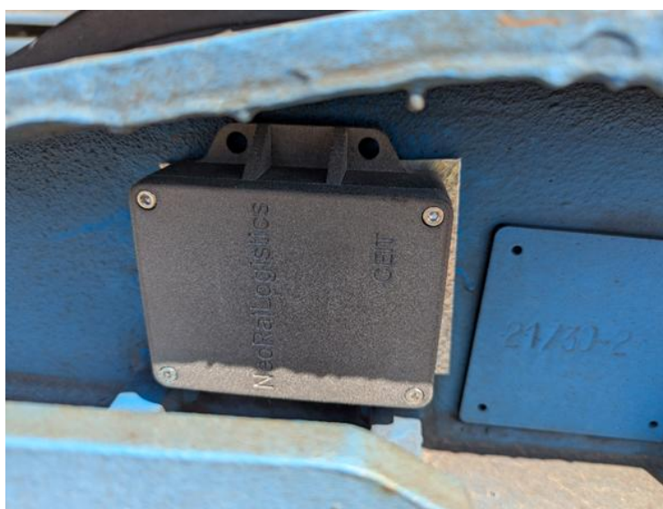
Figure 7.10 On-board unit attached to the metal plate
