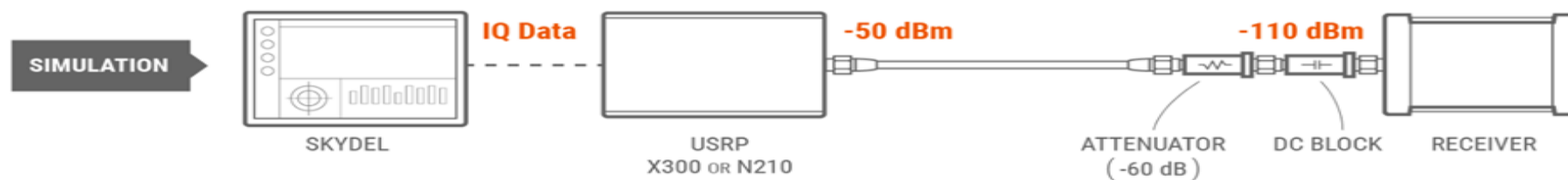
Propagation of the simulated GNSS signal from Skydel to the GNSS receiver
