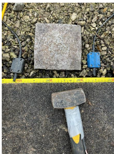
Figure 132 : Photograph of the hammer-type active seismic source on a metal plate between two geophones (black and blue).
