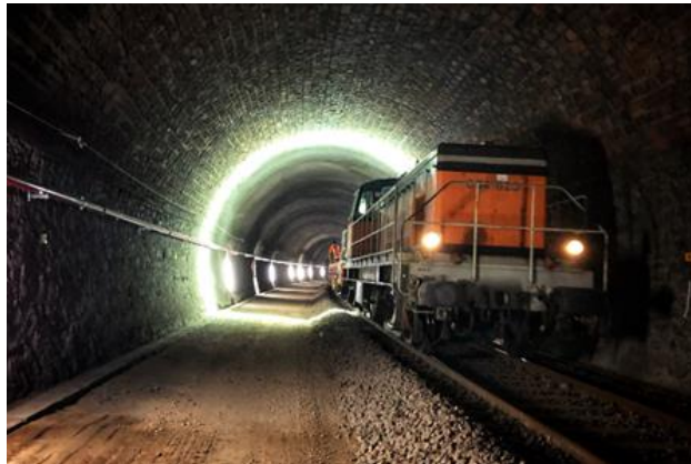
Figure 147. TS4 system from German company SPACETEC with line-scan cameras.
