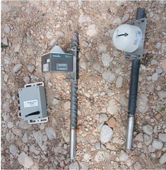
Figure 94. Type clinometers to be installed on the slope on rebar. Specifically, 14 clinometers of the same type as the one shown on the right of the image will be installed.
