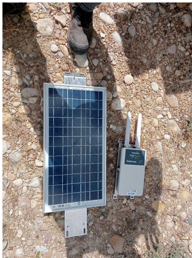
Figure 93. Detail of the Gateway and the solar panel to be installed on the catenary pole that is located in front of the unstable slope.
