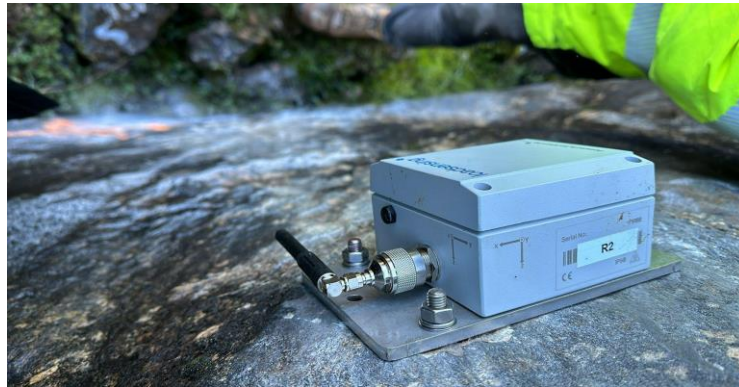
Figure 104. Tiltmeter installed on a rock.
