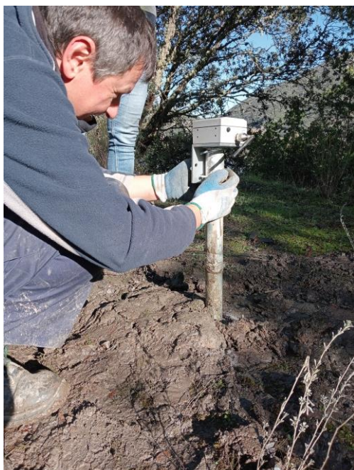
Figure 101. Installation of tiltmeter on a mast embedded in the ground.
