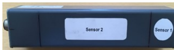
Figure 5-5: Inductive displacement sensor for switch rail position monitoring
