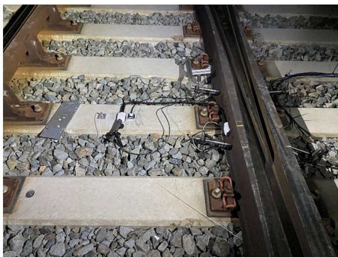
Figure 4-2: Installed multi-sensors in crossing panel for track quality and wing rail / crossing nose monitoring.
