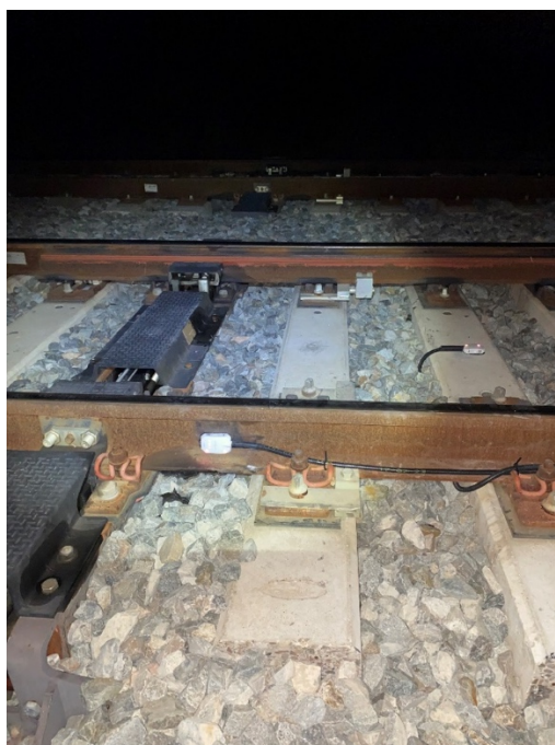
Figure 4-3: Multi-sensors installed in switch panel for track quality and switch rail / stock rail wear monitoring.
