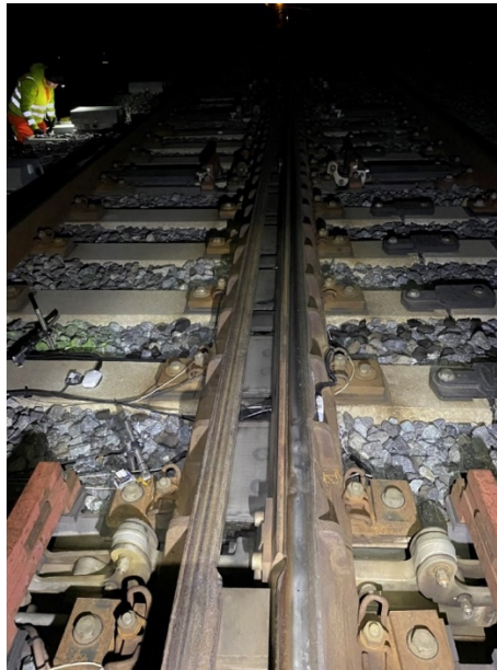
Figure 4-17: Multi-sensors installed in crossing panel for track quality and wing rail / swing nose monitoring.
