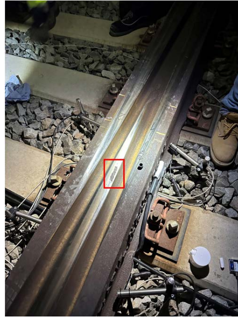
Figure 18-21: Picture from demonstrator turnout 9 months later in March 2024. The red box indicates initiated surface damage, a breakout, at the crossing nose running surface.
