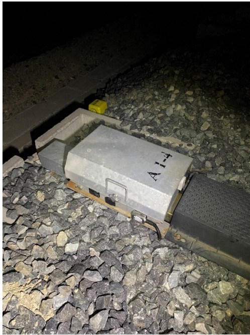
Figure 4-18: Analogue acoustic sensor installed on point machine casing for point machine monitoring
