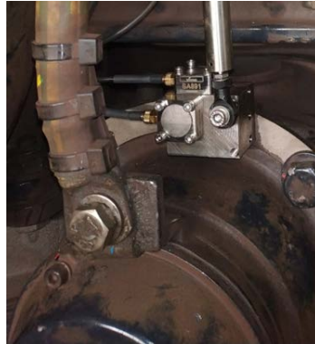
Figure 13-2. Installation of sensor in axle box for track geometry assessment.
