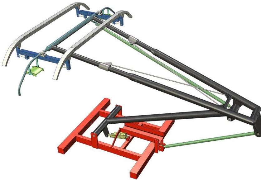
Fig. 13: Design for a generic Pantograph to be used for wind tunnel experiments and CFD
