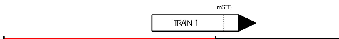
Figure 29: No shortening of front of Train Location due to clear TTD
