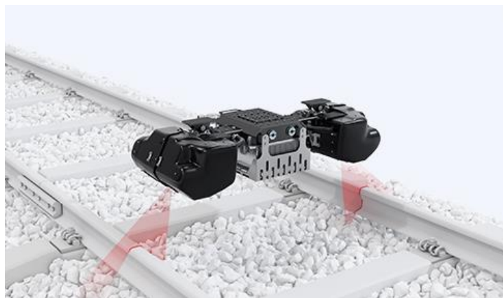
Figure 20 - Inertial-Based Track Geometry Measurement System (TGMS)
