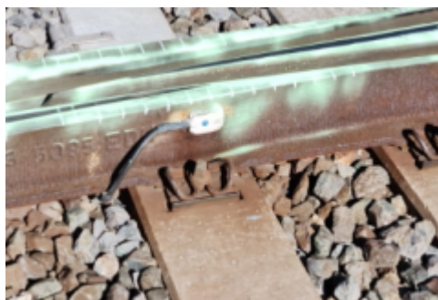
Figure 66: Multi-sensor system used for frog / switch rail monitoring
