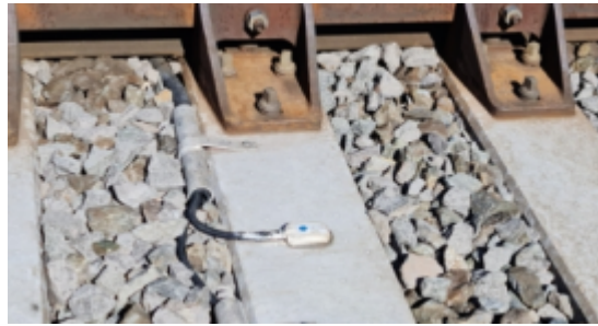
Figure 64: Multi-sensor system used for track quality monitoring
