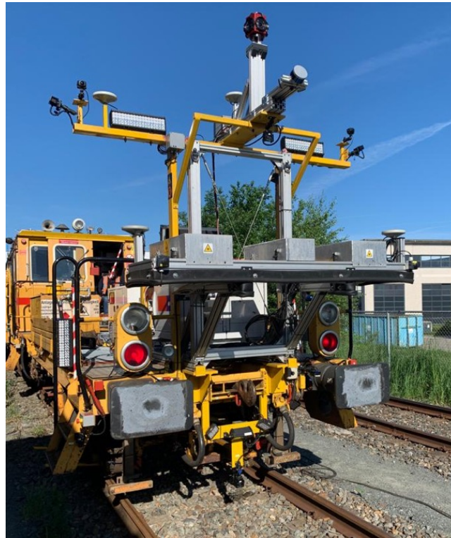
Figure 78: Measuring equipment on a re-used tamping machine
