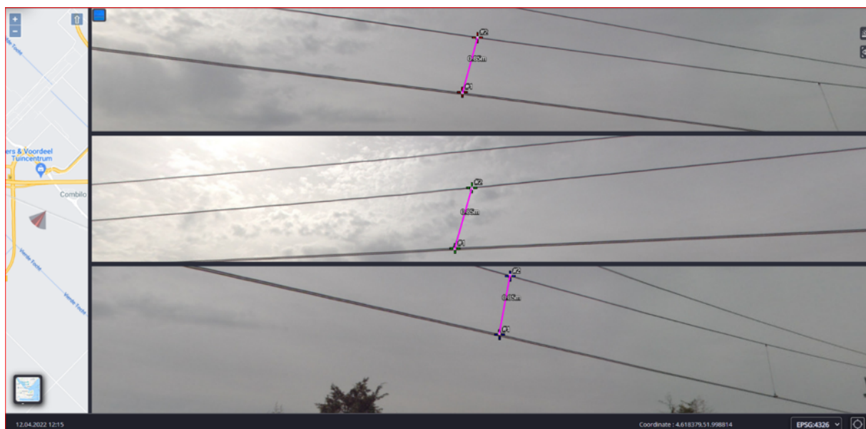
Figure 76: measuring length of hanging wires
