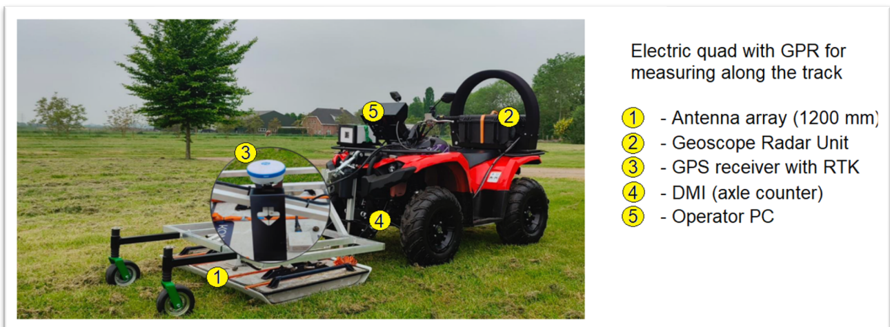
Figure 16: Radar system mounted of a vehicle
