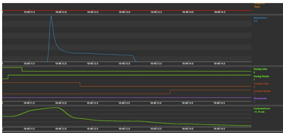
Figure 32: overview of measurements during a switch throw
