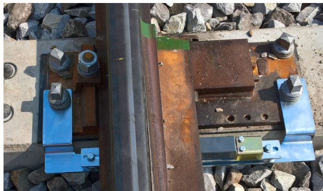
Figure 62: Example of the inductive position sensor utilised for switch assembly monitoring
