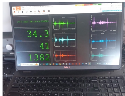
Figure 19: ABA connections datalogger & output on computer screen
