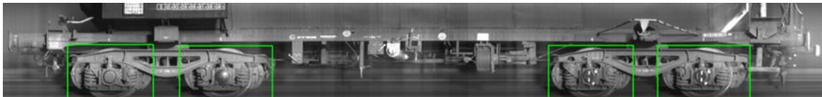
Figure 7.3 Object detection of the wheelset areas
