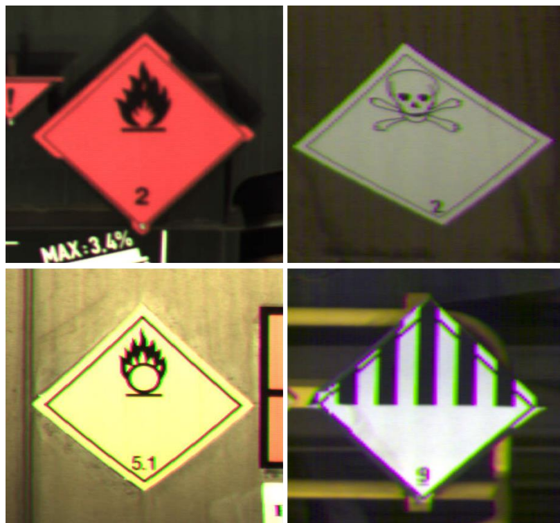
Figure 7.11 Examples of Hazmat signs, data provided by DB Cargo.
