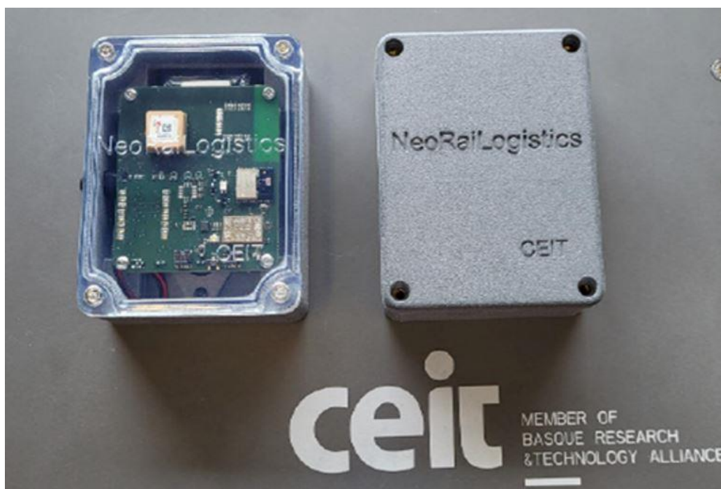
Figure 5.26 Wagon On Board unit (WOBU) and Sensor Node.
