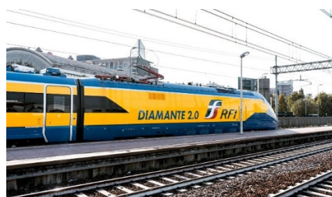
Dedicated MERMEC Vehicle for the digital twin High-speed Diamante 2.0 diagnostic train
