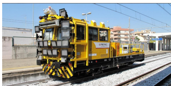
Dedicated MERMEC Vehicle for the digital twin High-speed Diamante 2.0 diagnostic train
