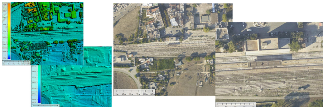
Aerial Surveying outputs sample data: Digital Terrain/Surface Models; Orthophotos
