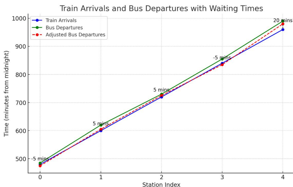
Figure 8 - Example of synchronization analysis of train arrivals and bus departures
