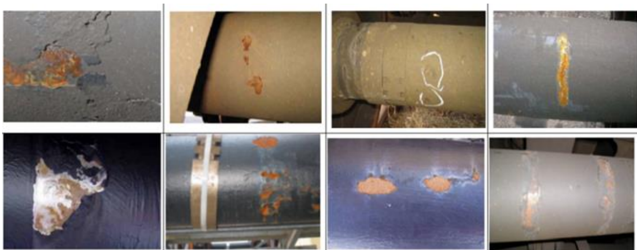
Figure 94: Coating damages on axles with corrosion
