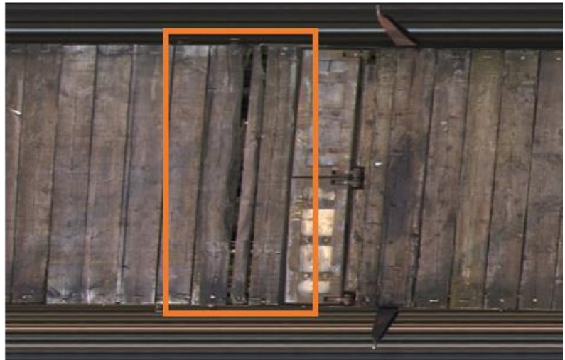
Figure 93: Tarpaulin cover with a cut (left) and damaged floor (right)
