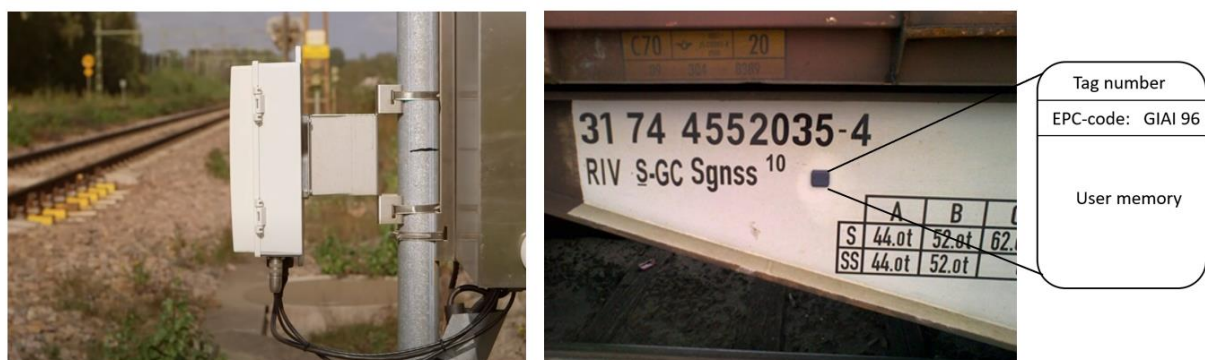
Figure 102: Rolling Stock identification through RFID antenna (right) RFID tag mounted on a wagon within a distance of 70 to 110 cm measured from top of the rail (left).
