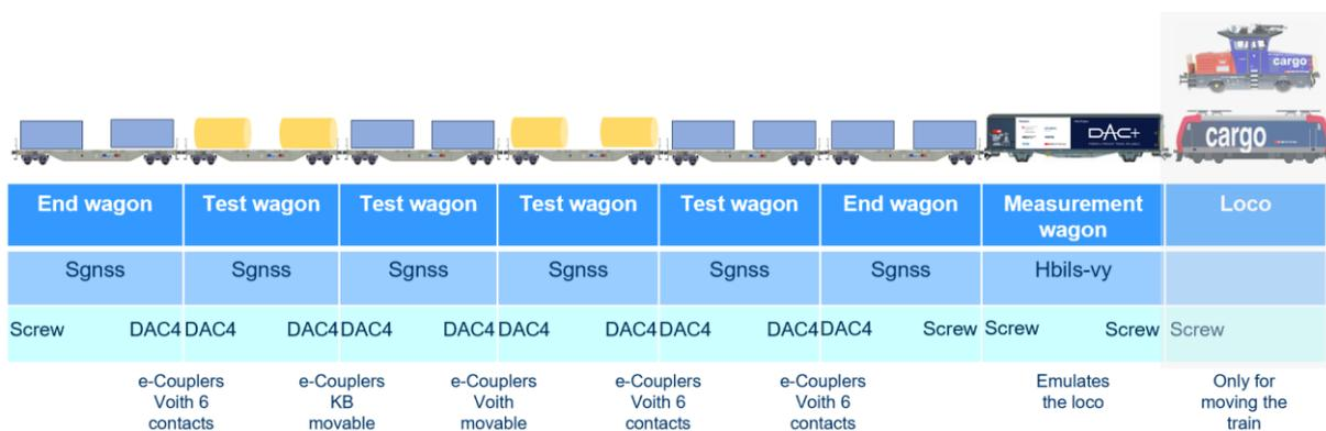
**Figure 2: Composition of prototype test train**
