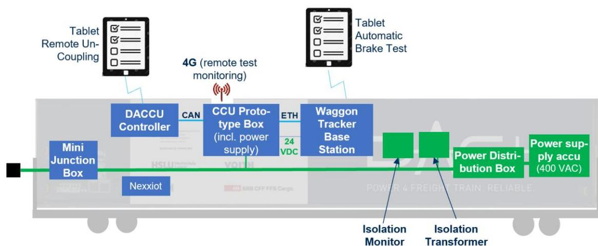
Figure 18: Equipment installed in the equipment and measurement wagon
