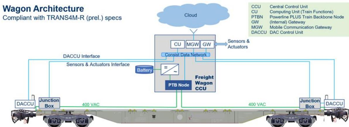
**Figure 4: Architecture of the PTB wagon power and communication system**
