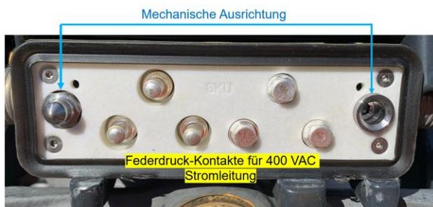
**Figure 14: Contact carriers and contacts of static e-couplers**
