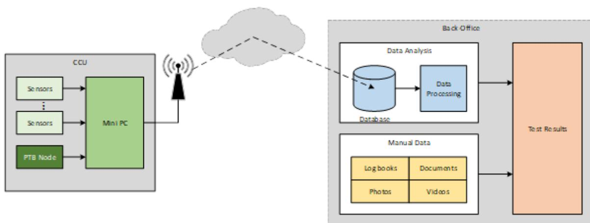
**Figure 8: Data acquisition and analysis system**
