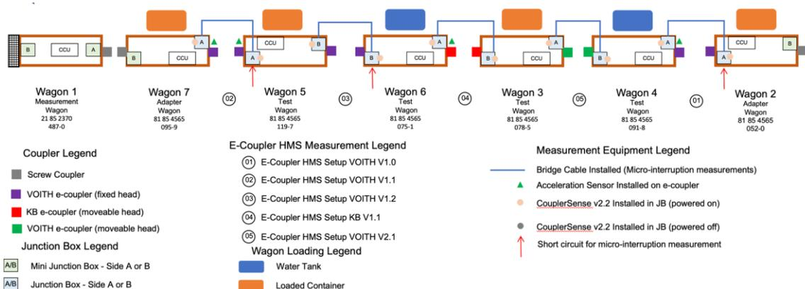
Figure 21: Test Drive Train Topology
