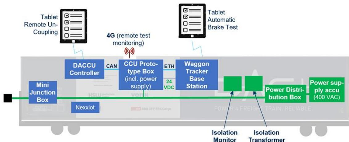
**Figure 6: System set-up Components in the equipment and measurement wagon**
