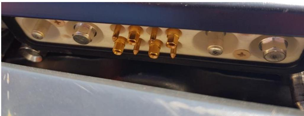
**Figure 12: Damaged Knorr-Bremse e-coupler**
