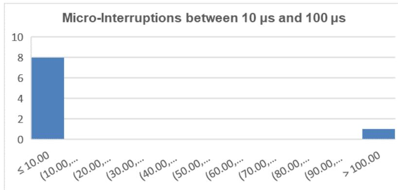
**Figure 11: Micro-interruptions on Voith e-coupler (fixed head)**
