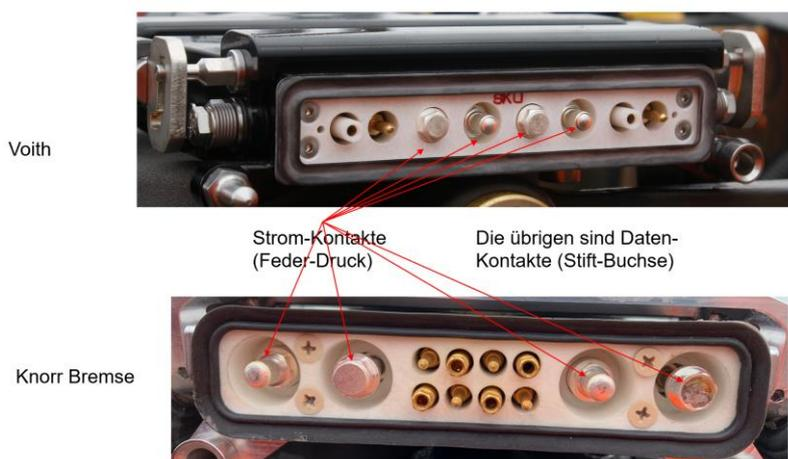
**Figure 15: Contact carrier and contacts of e-coupler with movable head**
