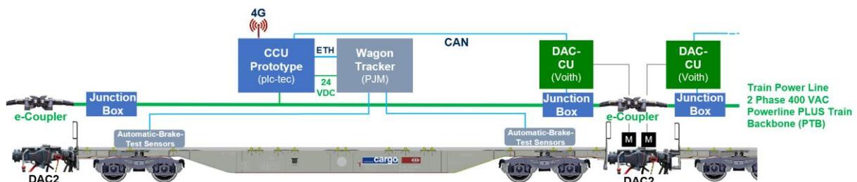
**Figure 5: Wagon test system set-up**
