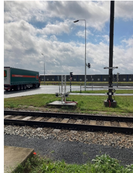
Photo: brake pad monitoring camera (left) and wagon number recognition camera (right)
