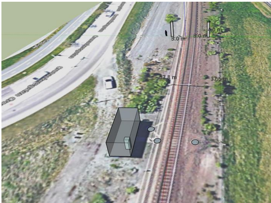
Figure 13. Positioning of poles, cabling and technical cabinet in Gothenburg.
