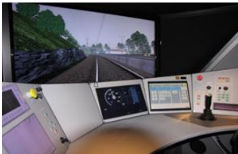
Figure 3: One hardware version of the VTI Train driving simulator.
