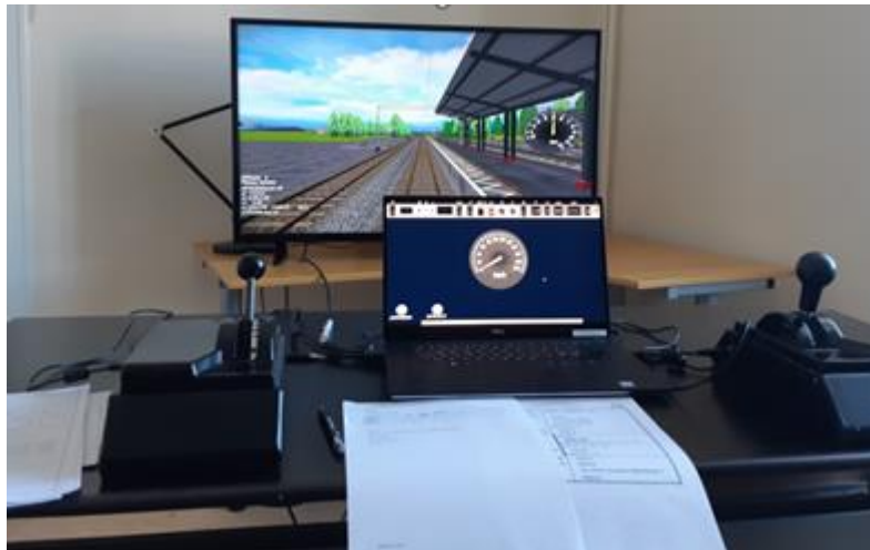
Figure 18: One hardware version of the VTI train driver simulator, used within the validation study.
