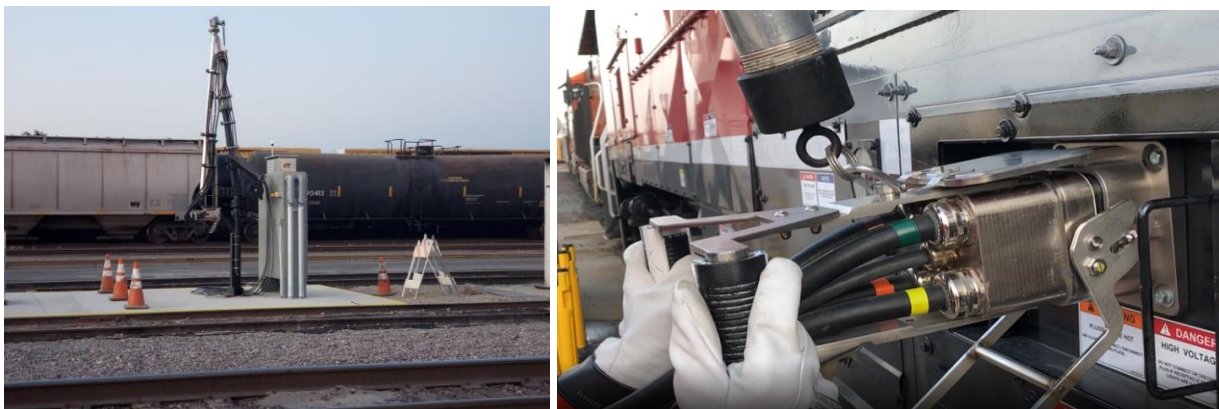
Figure 15: On the left, battery locomotive charging plug in Stockton (USA), on the right, charging plug connect to the battery locomotive.
