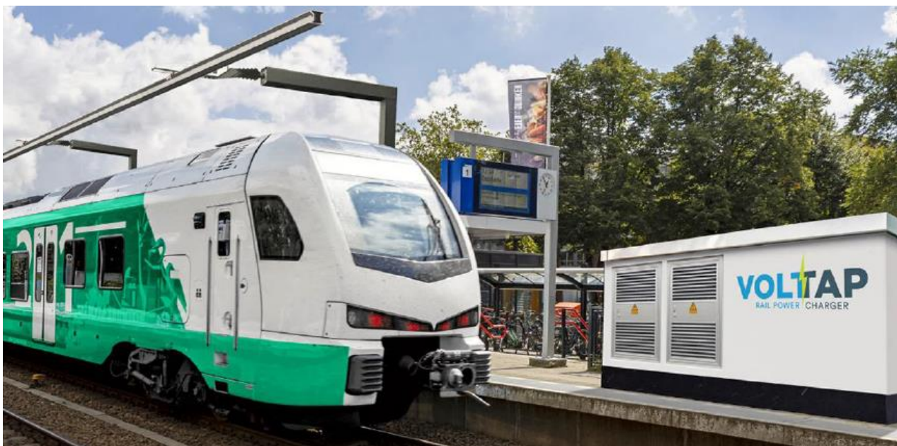
Figure 5: Example for fast charging via overhead current rail for catenary islands (VOLTAP system)
