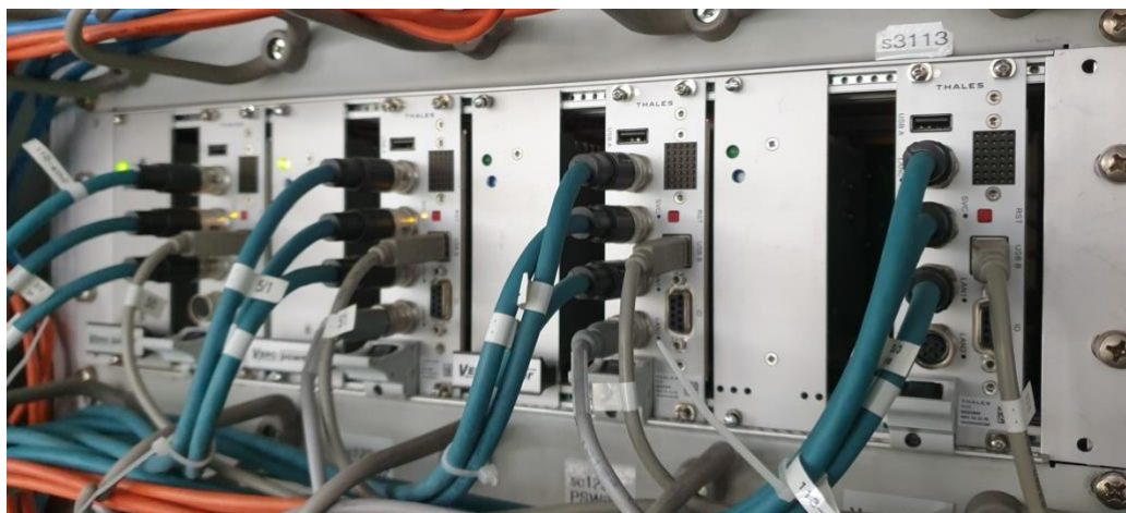
Figure 9: Sub-Rack with multiple CPU Boards
