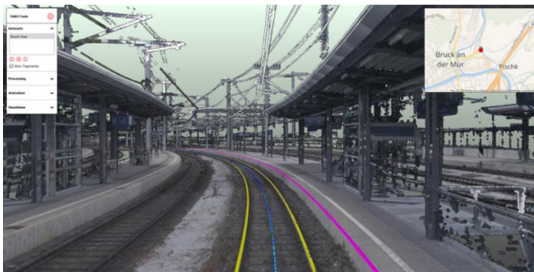
Figure 13: Example of extracted objects: platform, rails and track centreline
