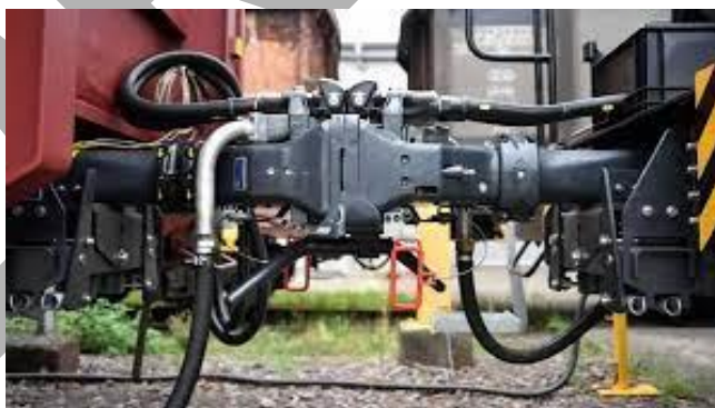
Figure 1 Representation of a DAC system
