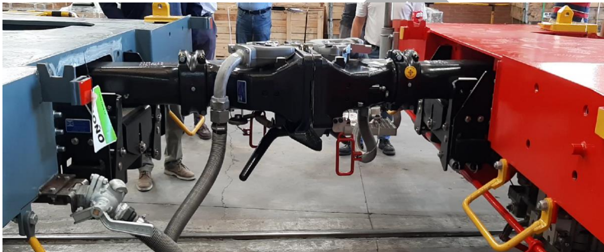
Figure 32 Coupling on a curved track
