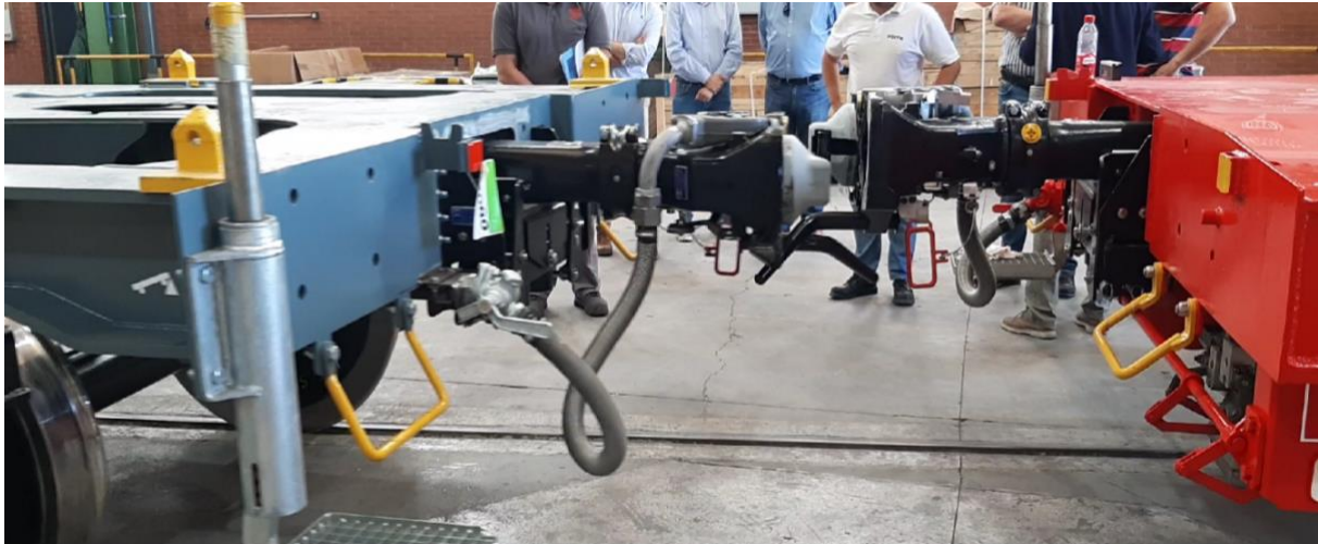
Figure 33 Coupling with a height difference between the AC's
