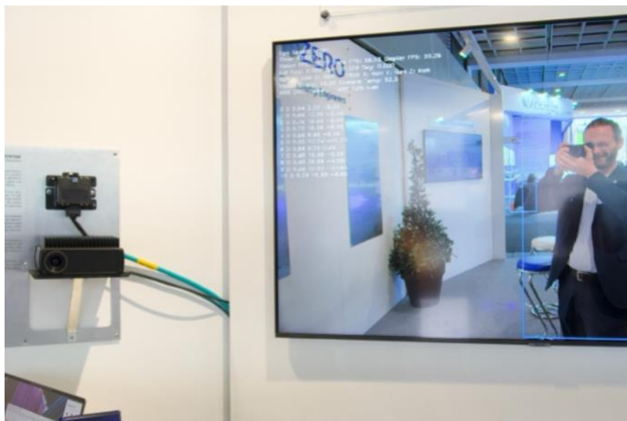
Figure 9 On-board perception system for automated shunting by m.ZERO (Photo: Fabian Acker, DB Cargo)
