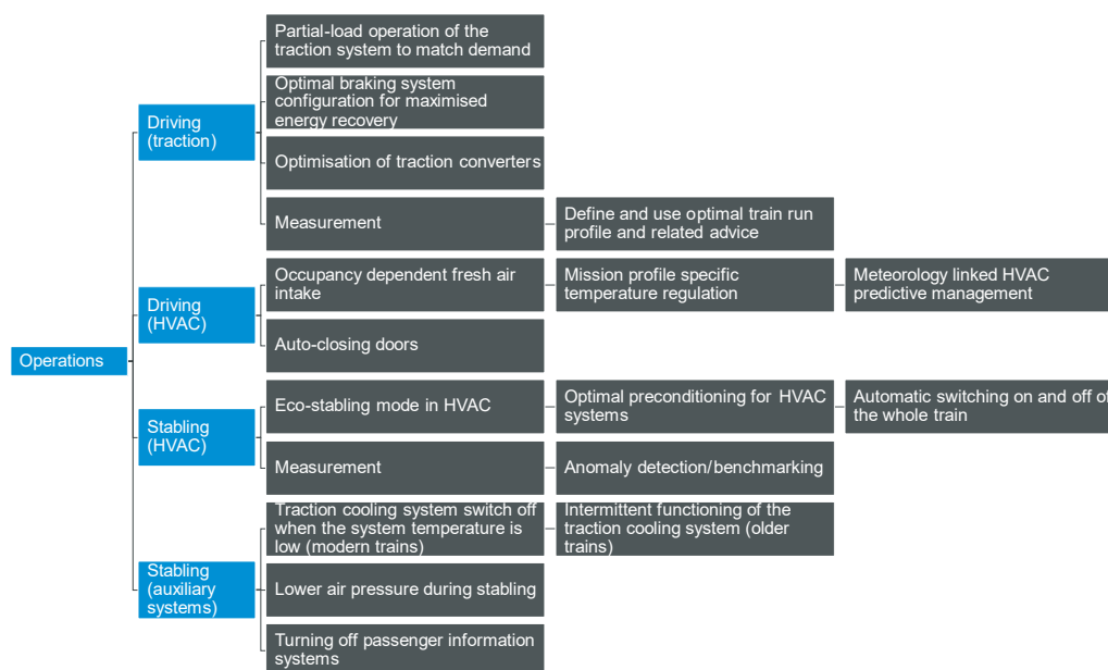
Figure 28: Overview of rolling stock software optimisation solutions as an outcome of the rolling stock and operations session of the UIC Energy Saving workshop
