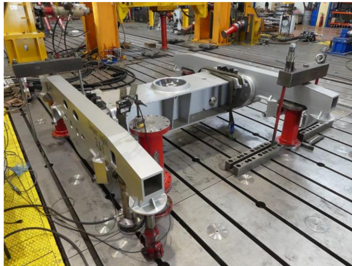
Realisation of torsion stiffness measurement
