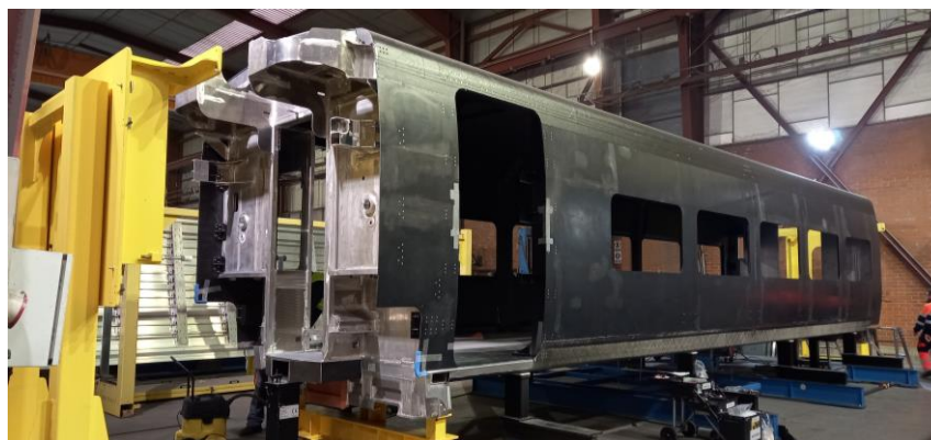
CFRP HS Carbody on the integration tool
