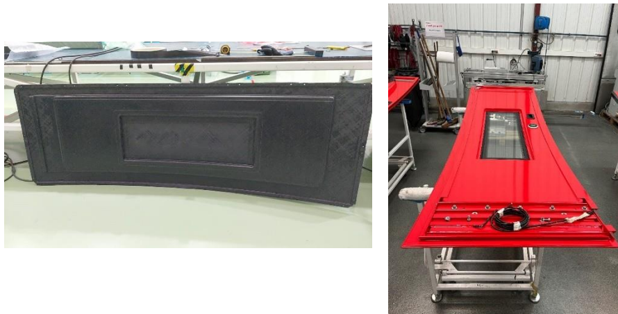
Composite part (left). Composite door leaf (right).
