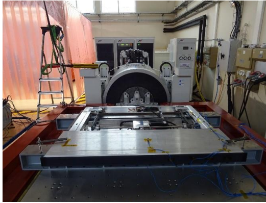
Bridging plate on the vibration test bench
