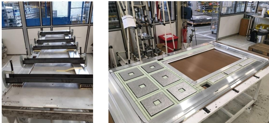
Bonding of the insulated pillars (left). Innovative filling material (right).
