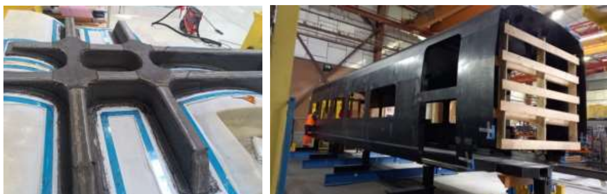
Component of headstock demo during manufacturing 2022 (left). High-Speed carbody demo prior to the final assembly 2022 (right).
