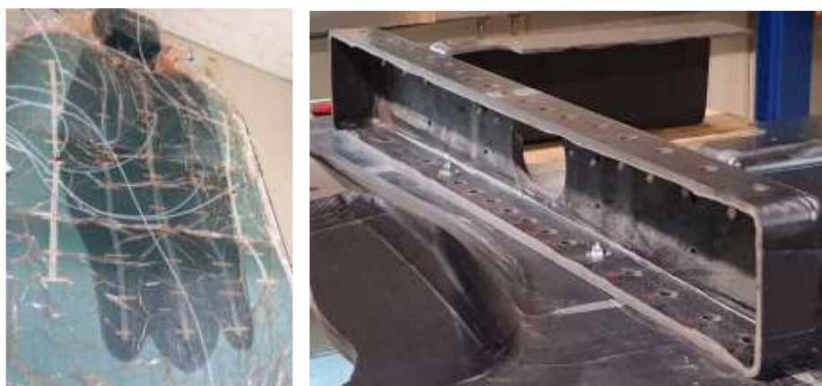
Infusion process for component manufacturing 2022 (left). Component under machining process 2022 (right).
