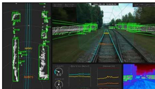
GUI visualizing the CAS system (top-right: camera image, left: abstracted top view, bottom-center: overview dashboard, bottom-right: infrared camera)
