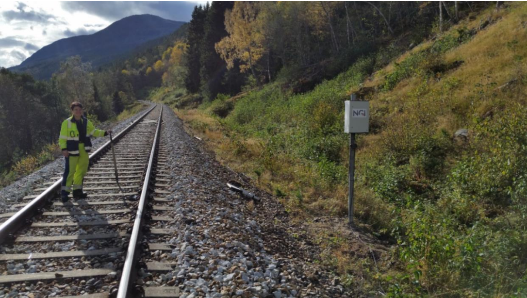
warning system test site, showing an electronics cabinet housing two relay radio units with directional yagi antennas
