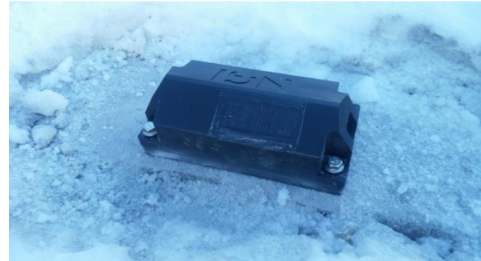
self-contained sensor units, which contains the sensors, data acquisition unit, radio module, antenna, and battery.
