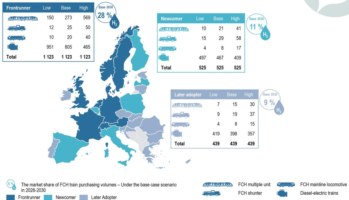
**Figure 3:** FCH train market outlook for 2028-2030 in standard units [vehicles, train segments for Multiple Units].
