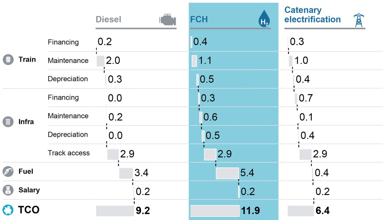
**Figure 21:** TCO analysis of different technological options for Frankfurt (Oder) - Hamburg (in EUR/km)<sup>67</sup>
