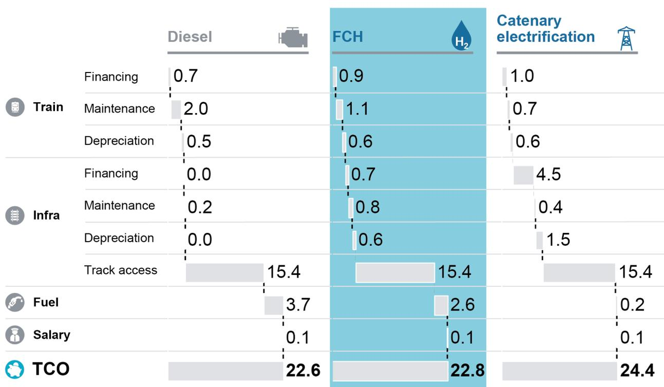
Figure 17: TCO analysis of different technological options for Tallinn – Narva (in EUR/km).
