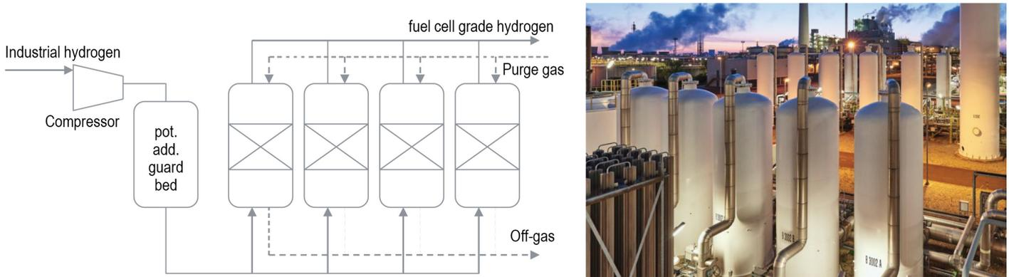
**Figure 27:** Process flow PSA (simplified) and PSA installation.
