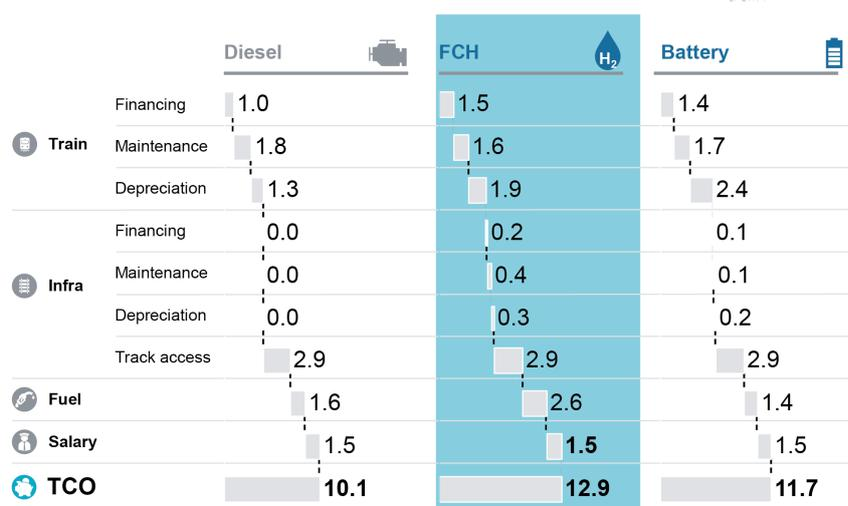
**Figure 11:** TCO analysis of different technological options for Hamburg-Billwerder (in EUR/km)<sup>40</sup>
