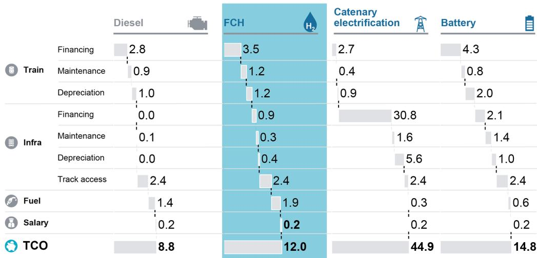
**Figure 7:** TCO analysis of different technological options for Brasov - Sibiu (in EUR/km)
