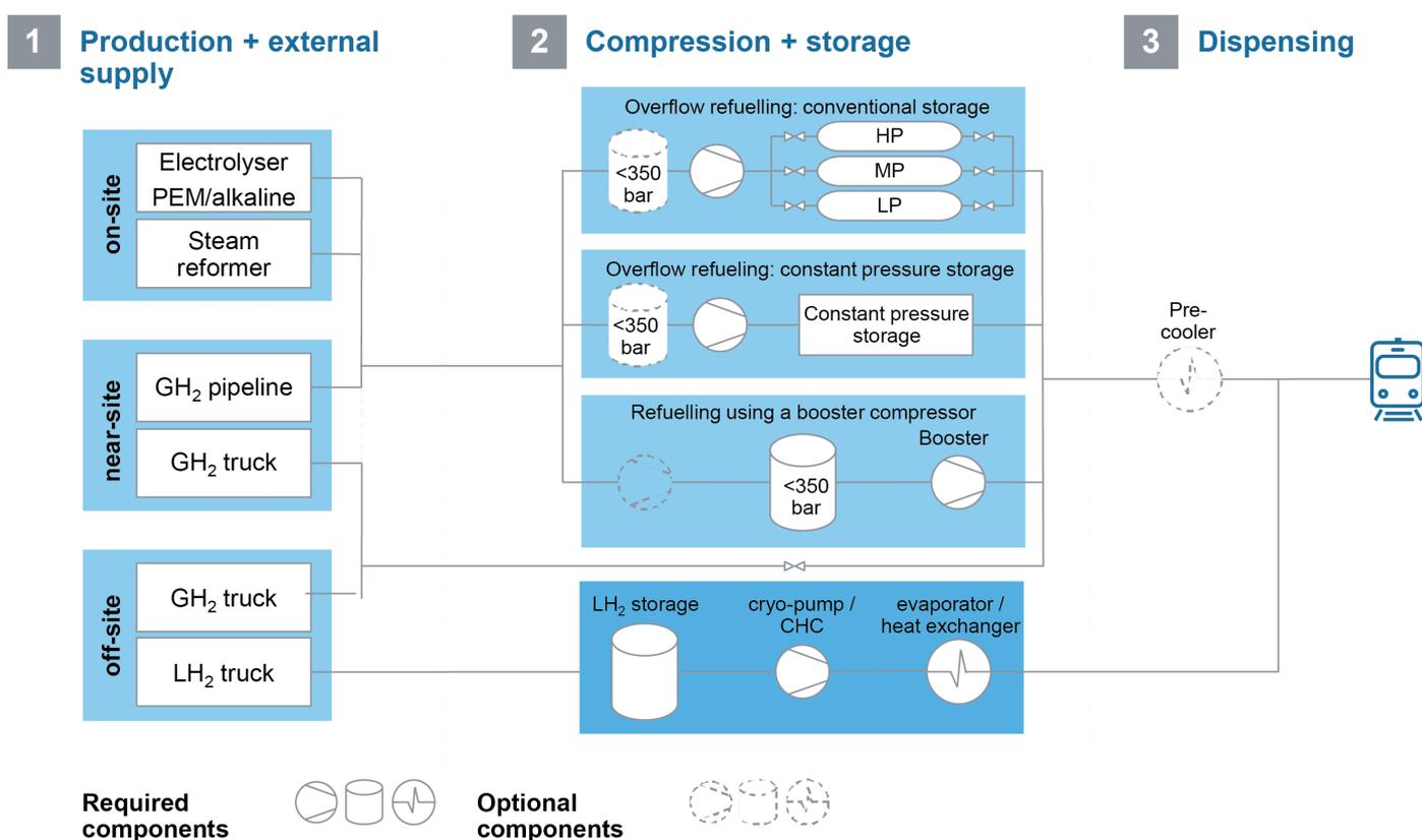
Figure 26: Schematic overview of HRS pathways<sup>82</sup>
