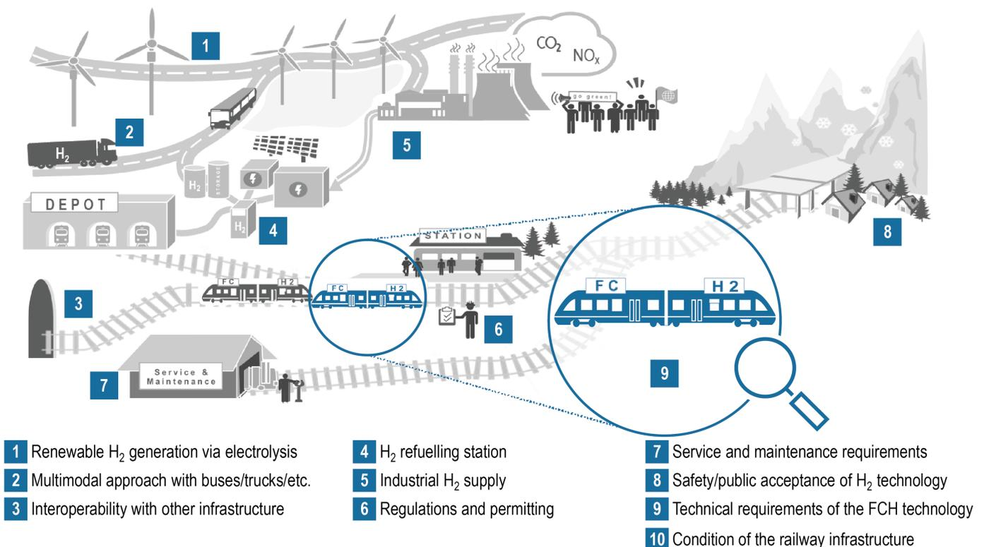
**Figure 23:** Schematic of FCH train eco-system including selected focus topics.
